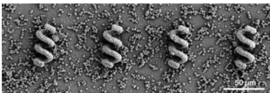
Figure 8: Electron micrograph of a micro helices prepared by lithographic approach. [39]
