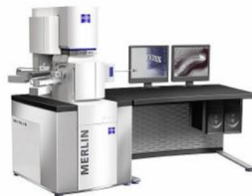
Figure 11: SEM instrument of high resolution, from Electron Microscopy facilities of Universitat Autònoma de Barcelona (UAB)
