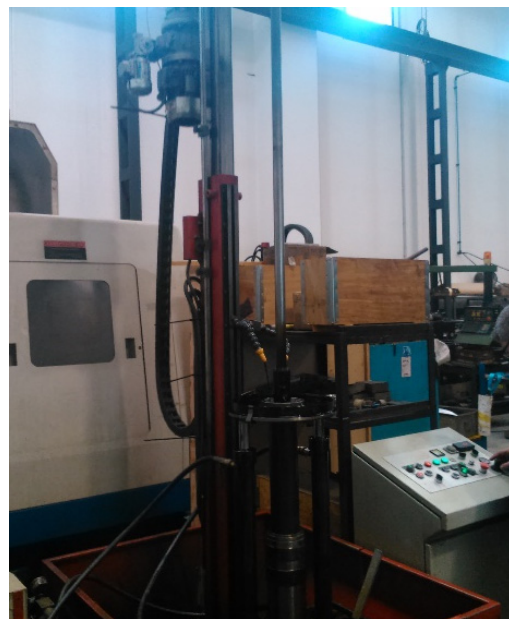
Figure 1. Industrial honing machine used in the experiment.
