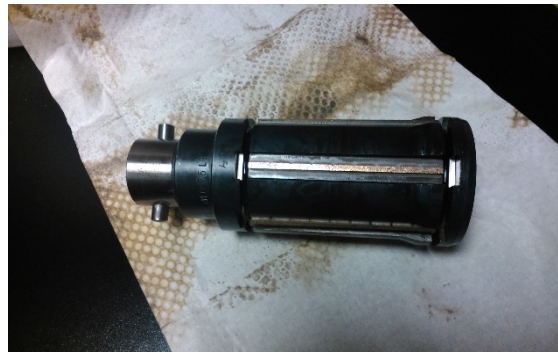
Figure 2. Honing head used in the experiment.
