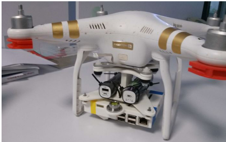
Fig 1. Payload mounted on a DJI (Phantom IV) quadcopter. Housing can bear one or two cameras.
