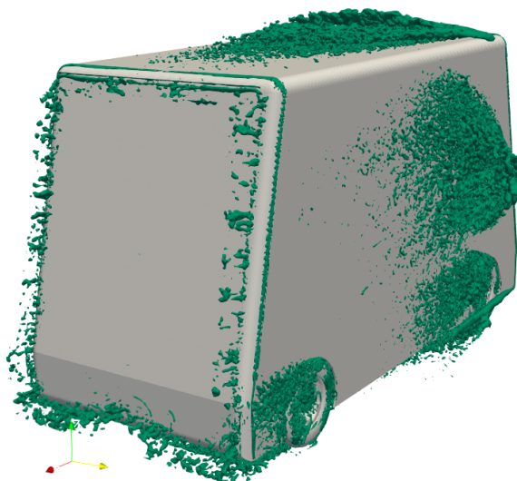
Figure C.95: Rear isometric view of the Q-criteria (value q = 2000 \text{ s}^{-2} ) of sensor position f and type small puck
