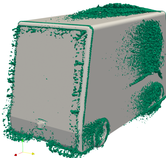
Figure D.32: Rear isometric view of the Q-criteria (value q = 2000 \text{ s}^{-2} ) of sensor layout coded: a_S_g_S_i_S
