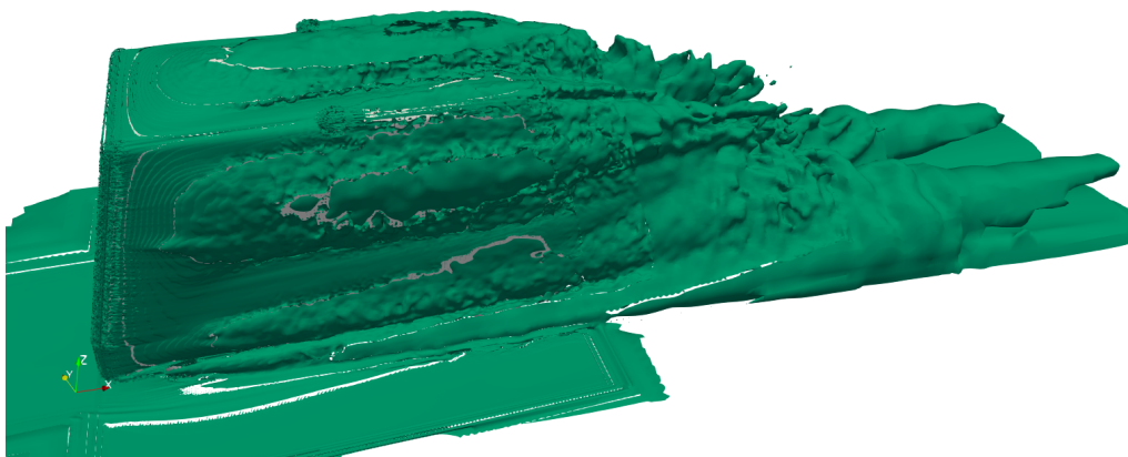
Figure C.197: Side view of the vorticity (value |\omega| = 10 \text{ s}^{-1} ) of sensor position I and type big puck
