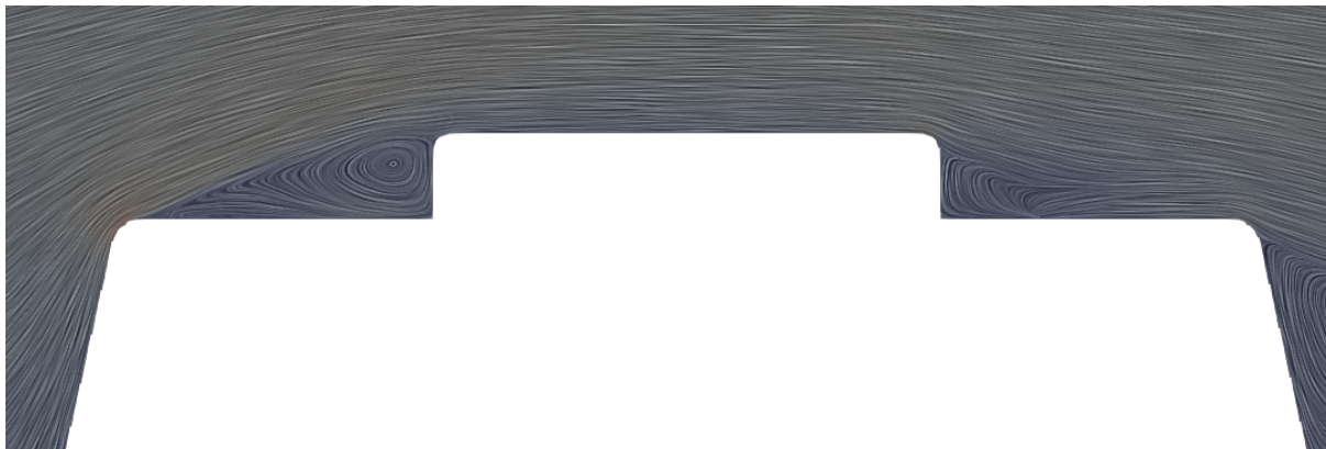
Figure 4.11: Streamline representation of the aerodynamic working principle of the top-located box shaped sensor. It blocks the turbulence in front of it and allows the attachment of the flow on its top surface
