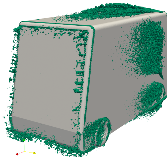
Figure C.5: Rear isometric view of the Q-criteria (value q = 2000 \text{ s}^{-2} ) of sensor position a and type small puck
