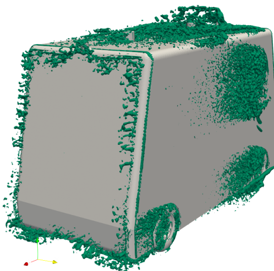
Figure D.41: Rear isometric view of the Q-criteria (value q = 2000 \text{ s}^{-2} ) of sensor layout coded: b_B_c_S_I_S
