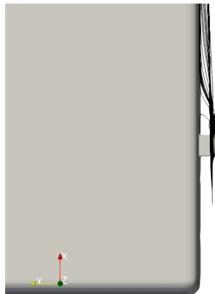
(d) Top view of streamlines impacting at the most outer part the big puck sensor of position g
