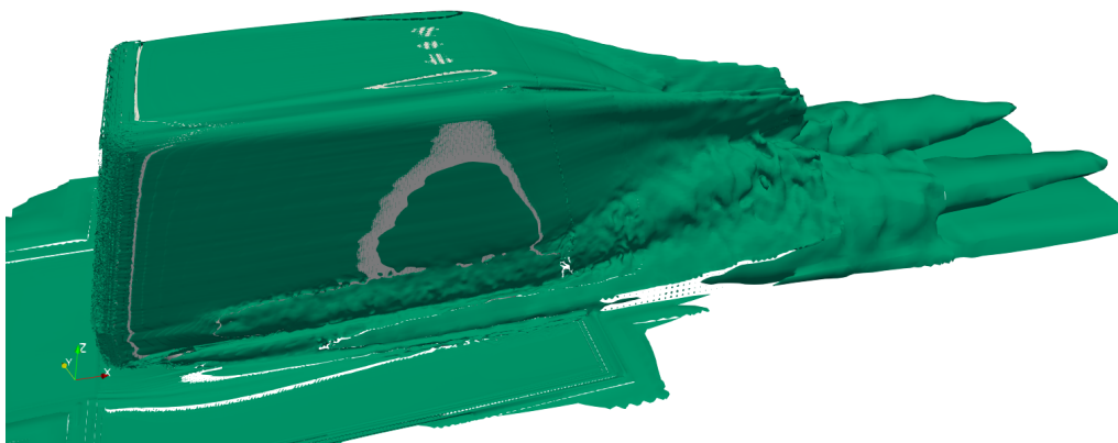
Figure B.36: Side view of the vorticity (value |\omega| = 10 \text{ s}^{-1} ) of design modification: rounding of 197.8 mm
