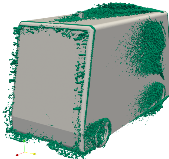
Figure C.50: Rear isometric view of the Q-criteria (value q = 2000 \text{ s}^{-2} ) of sensor position b and type big puck
