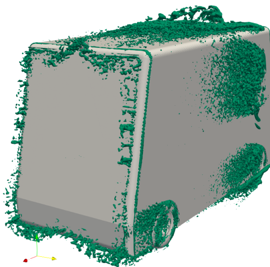
Figure C.59: Rear isometric view of the Q-criteria (value q = 2000 \text{ s}^{-2} ) of sensor position c and type small puck
