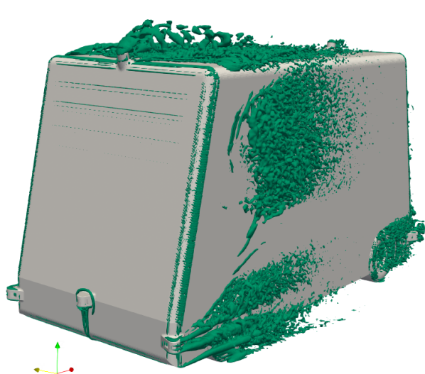
Figure D.47: Front isometric view of the C_p of sensor layout coded: a_S_c_S_h_S_i_S
