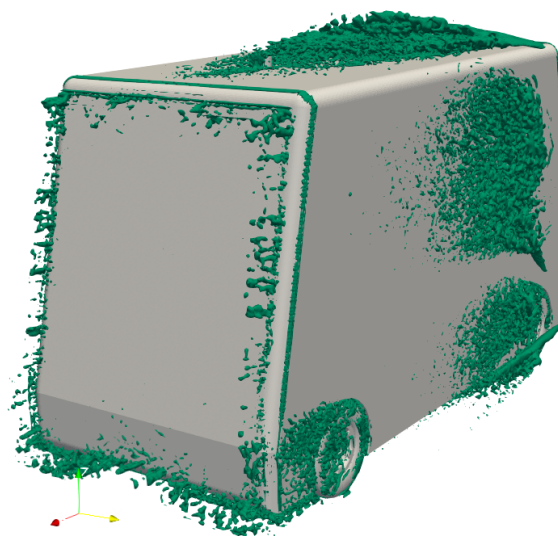
Figure C.41: Rear isometric view of the Q-criteria (value q = 2000 \text{ s}^{-2} ) of sensor position b and type small puck
