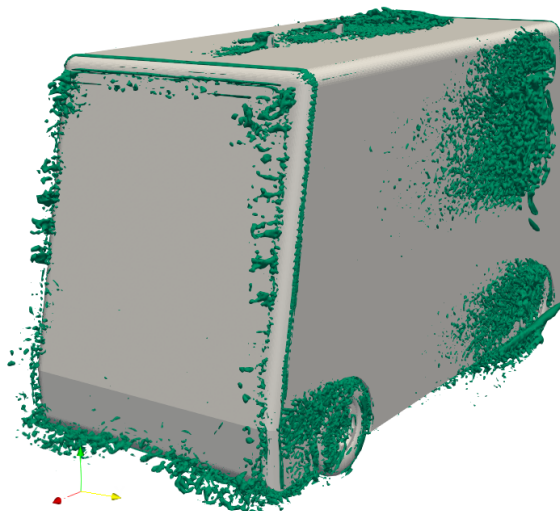
Figure D.23: Rear isometric view of the Q-criteria (value q = 2000 \text{ s}^{-2} ) of sensor layout coded: a_S_b_S_k_S
