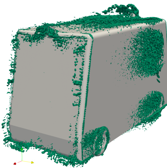
Figure C.68: Rear isometric view of the Q-criteria (value q = 2000 \text{ s}^{-2} ) of sensor position c and type big puck
