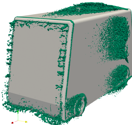
Figure C.14: Rear isometric view of the Q-criteria (value q = 2000 \text{ s}^{-2} ) of sensor position a and type big puck
