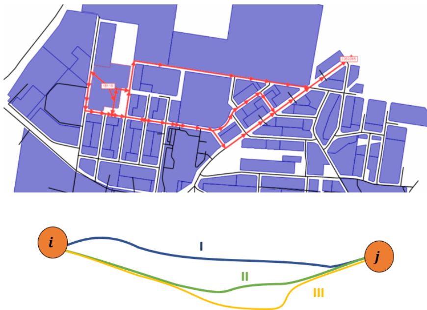
Figure 6.2: Path set ( \mathcal{P}_{ijr} ) for a selected origin and destination in the network
