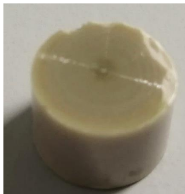
Figure 70. Facing in the 12\text{Ce-ZrO}_2 CIP sample.
