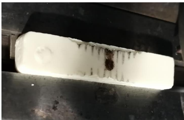
Figure 71. Milling footprints on the 12\text{Ce-ZrO}_2 sample.
