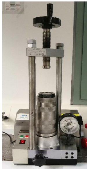
Figure 29. Cold Isostatic Pressing machine used in this bachelor's degree project.
