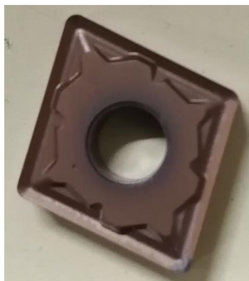
Figure 31. Tools used on the lathe CNMG120408 SM.
