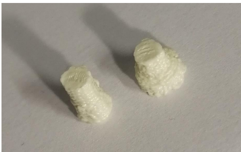
Figure 68. 12Ce-ZrO implant breakage.
