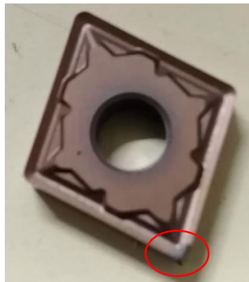
Figure 69. Tool CNMG120408 with broken tip when attempting to machine
