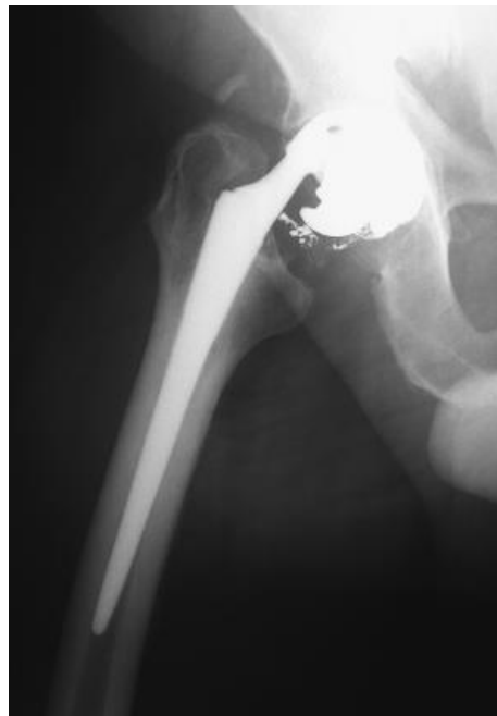
Figure 18. Radiograph of fractured 3Y- ZrO_2 head (29)..
