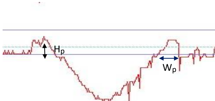
Figure 48. Schematization of the parameters measured in the confocal
