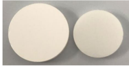
Figure 26. Sample before and after the sintering process (left and right, respectively)
