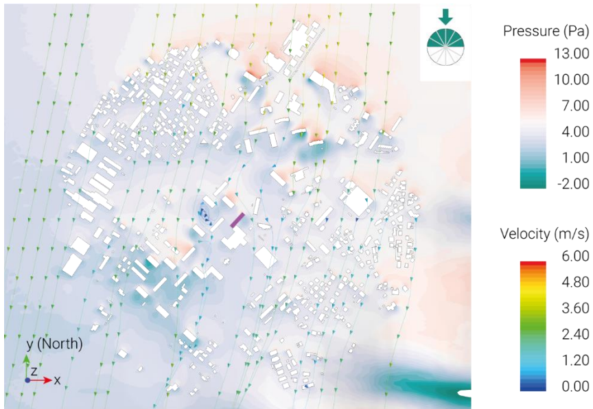
Figure 5.15 – Top view of pressure levels and streamlines: incoming wind from North (-y)
