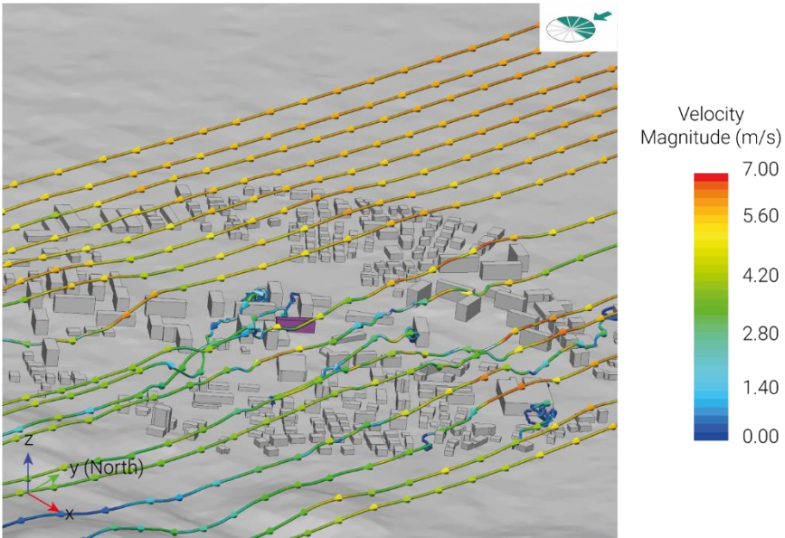
Figure 8.31 - Axonometric view of streamlines in the urban fabric: incoming wind from North (-y)
