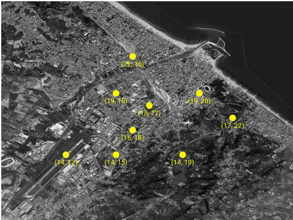
Figure 4.6 - Extraction points of the virtual anemometers
