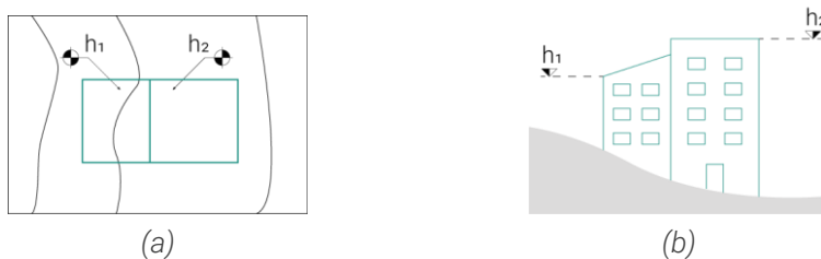
Figure 5.4 - Elevation of buildings in the CTR in plan (a) and section (b) view
