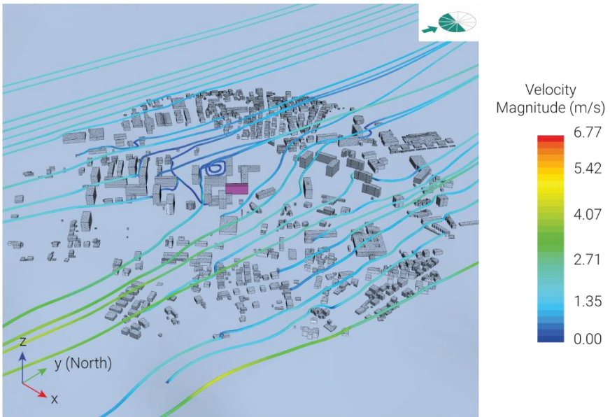
Figure 5.25 - Axonometric view of streamlines in the urban fabric: incoming wind from South (+y)
