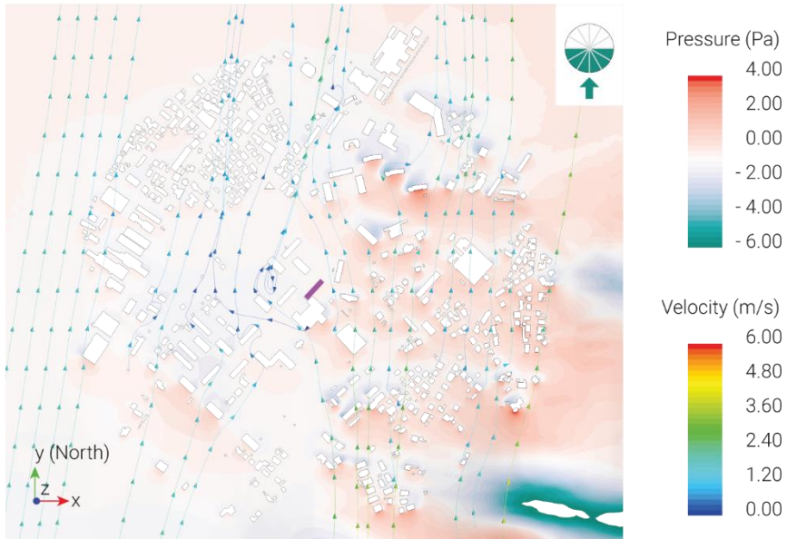
Figure 5.23 – Top view of pressure levels and streamlines: incoming wind from South (+y)
