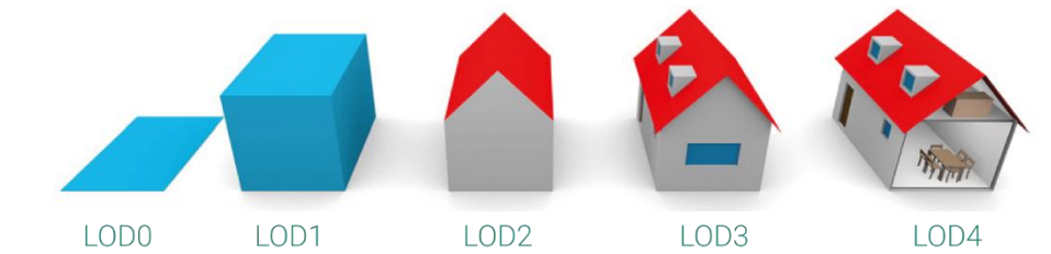
Figure 1.8 - Representation of the five LODs (figure from [36])
