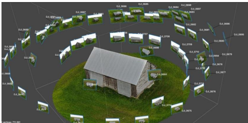
Figure 1.7 - Photogrammetry technique to reconstruct objects in 3D (figure from https://bitfab.io/blog/photogrammetry/ )
