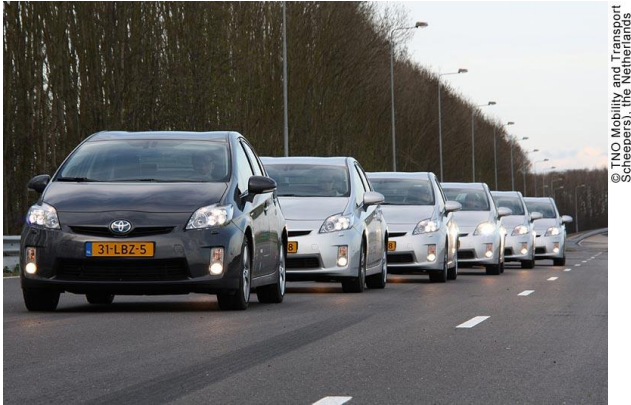
Figure 2 : CACC 6-car platoon, as part of the Connect and Drive Project. Source: Federal Highway Administration Research and Technology.
