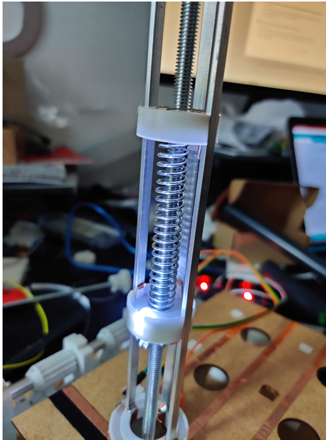
Figure 21: Weight sensor after replacing the laser by a white led
