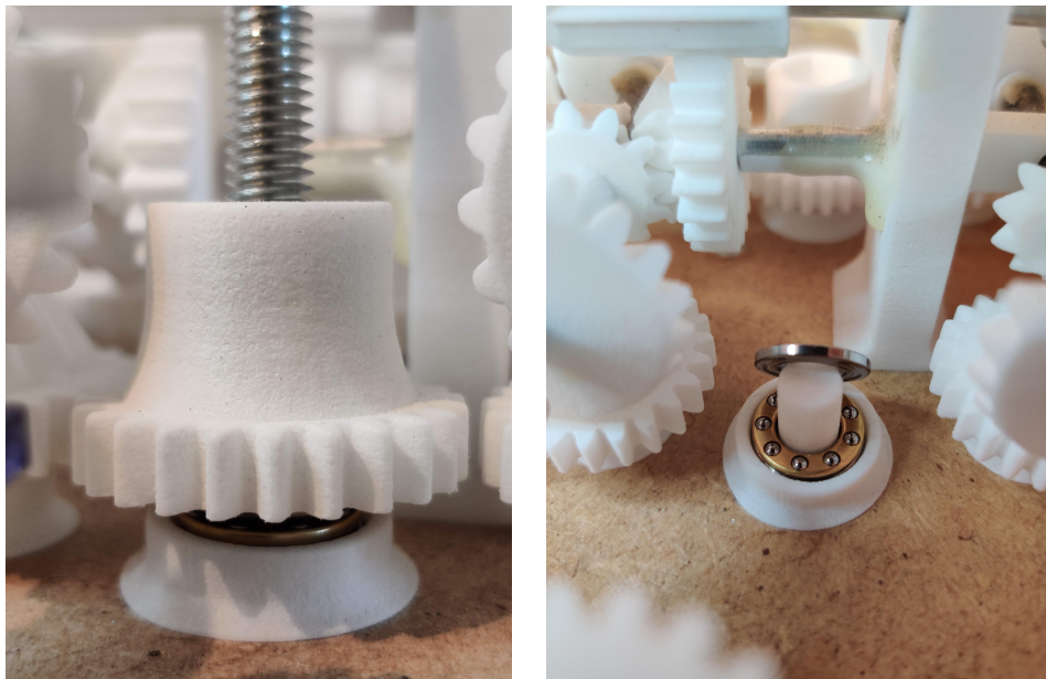
(a) Lift's gear and thrust bearing
