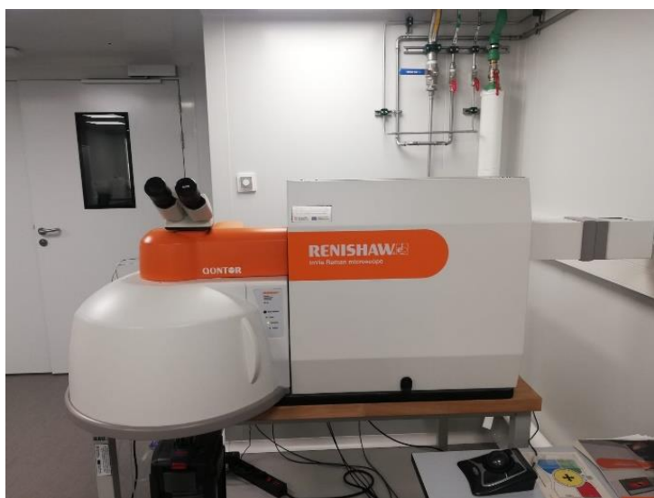
Figure 4.5. Image of the Confocal Raman Microscope inVia™ Qontor® from Renishaw (own elaboration).
