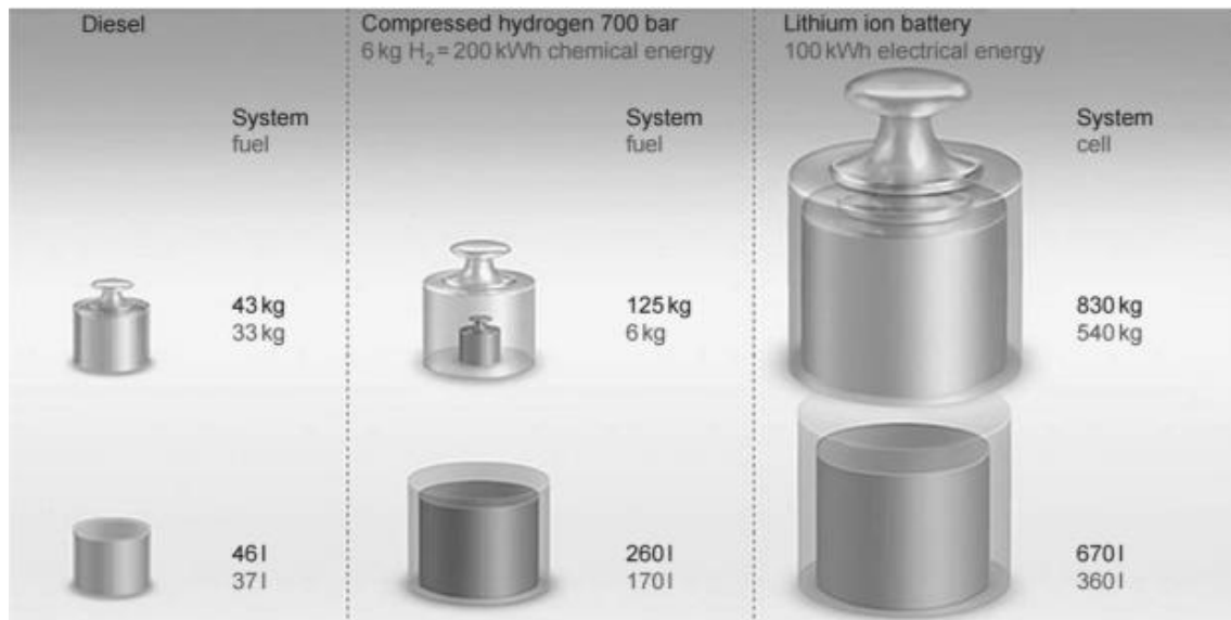
Figure 7.14. Scheme of the comparison of weight and volume for diesel, hydrogen and an electric battery, to obtain an autonomy of 500 km (Wilberforce et al. , 2017).
