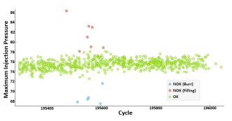
Fig. 3. Maximum injection pressure parameter representation.
