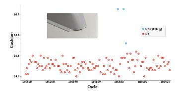
Fig. 1. Production cycle with NOK parts associated with filling problems (blue).
