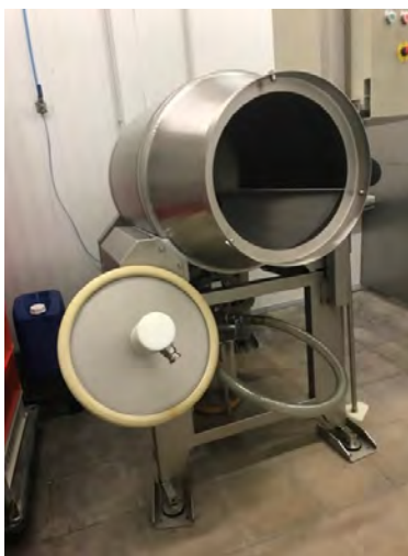
Figura 12: Bombo Lutetia al vuit: model 17608 ,7rpm
