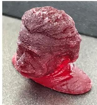
**Figure 6.** A 3D printed bust of Albert Einstein. The clearly visible layers had a thickness of 0,075mm each.
