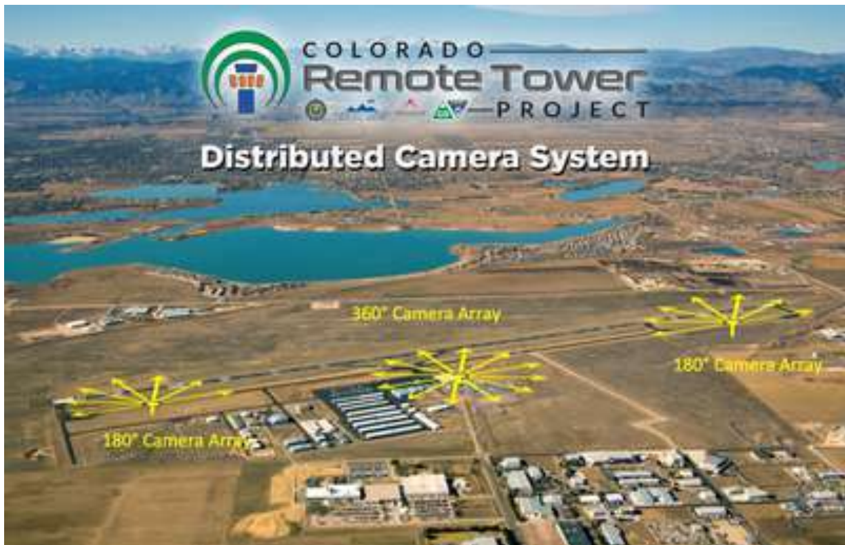
Figure 3.9: Cameras Layout at Northern Colorado Regional Airport Source: Colorado Dept. of Transportation [51]
