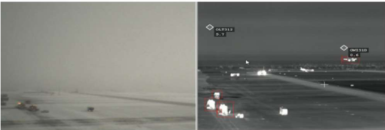
Figure 3.19: Traditional view under poor visibility conditions (left) compared to the same scene enhanced by virtual tower with infrared view and object detection and tracking tools (right).
