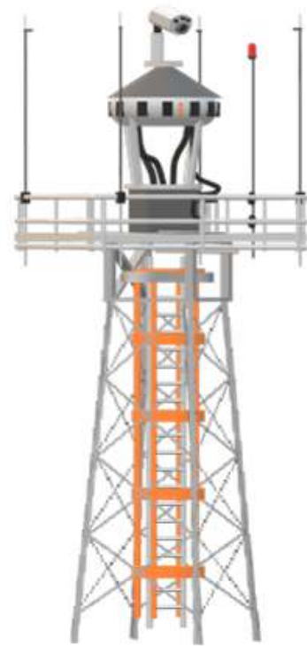
Figure 3.4: Remote Camera Tower
