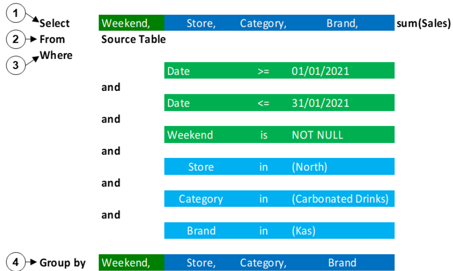
Figure 3.1: Basic SQL query structure, corresponding to question: “How much carbonated drinks of Kas brand the company sold every weekend during the first quarter of the year at the North store?”.
