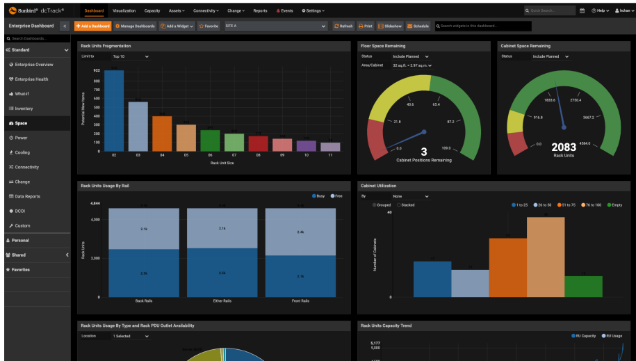
Figure 7: SunbirdDCIM example capacity dashboard. Source: SunbirdDCIM [6]
