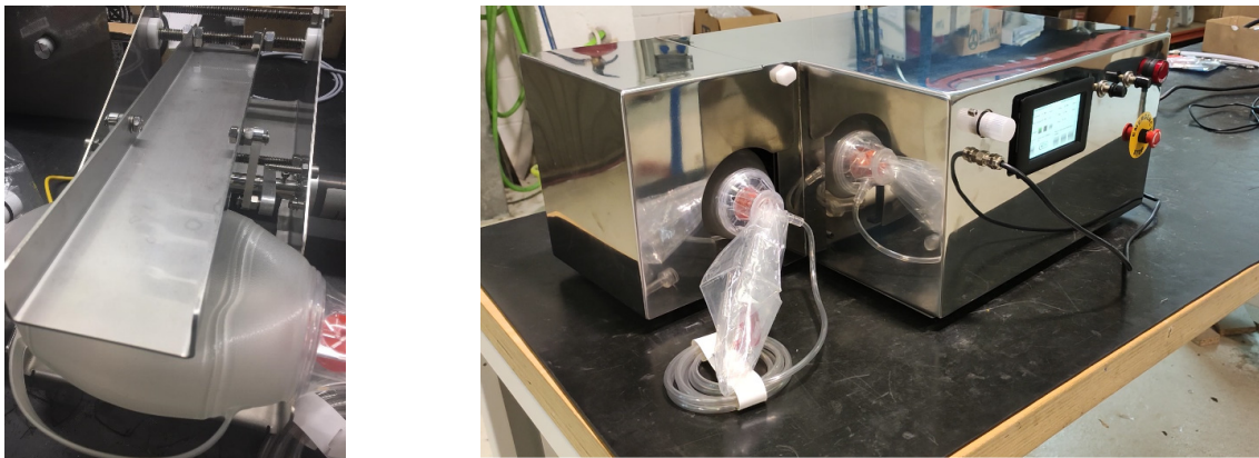
Figure 11. (a) respirator without the protective housing; and (b) complete system with the housing.
