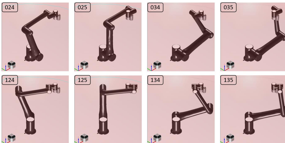
Figure 4.3.4 – Pose of robot can be in 8 different configurations: 024: RIGHTY, ABOVE, NOFLIP; 025: RIGHTY, ABOVE, FLIP; 034: RIGHTY, BELOW, NOFLIP; 035: RIGHTY, BELOW, FLIP; 124: LEFTY, ABOVE, NOFLIP; 125: LEFTY, ABOVE, FLIP; 134: LEFTY, BELOW, NOFLIP; 135: LEFTY, BELOW, FLIP (source: own).
