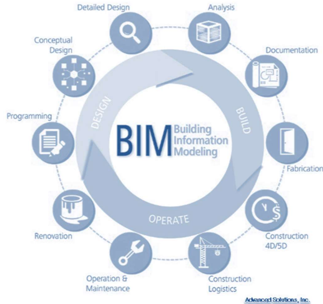
Figure 4: Life cycle in the Building Information Modeling methodology. Source: Advanced Solutions, Inc. [15].
