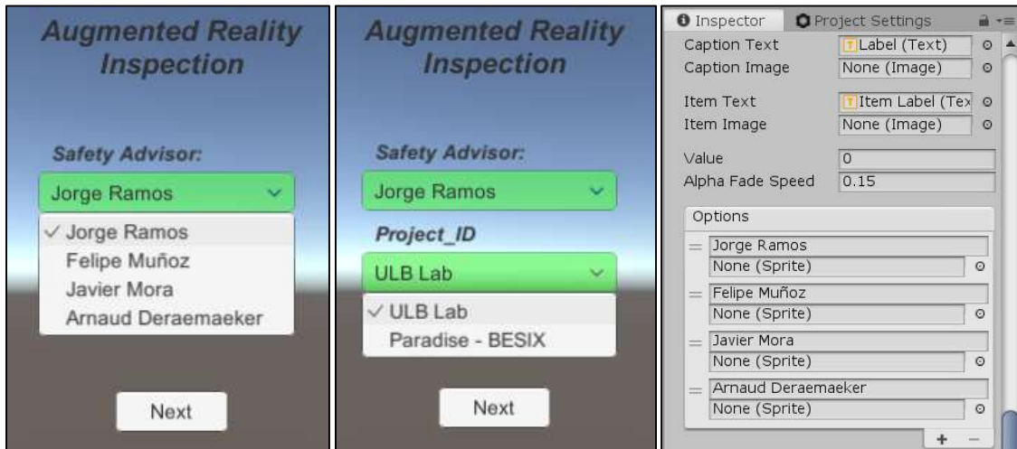
Figure 38: Overview of the dropdown menus in the first UI (1 st and 2 nd pictures) and configuration of the options in the inspector window for the inspector's name (3 rd picture).
