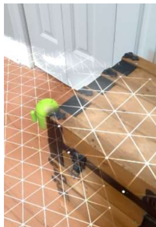
Figure 8: A digital object being covered by a real object. Source: Google, ARCore.
