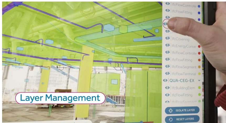
Figure 12: Layer Management interface in the AR application developed by Genie Vision. Source: Genievision.com
