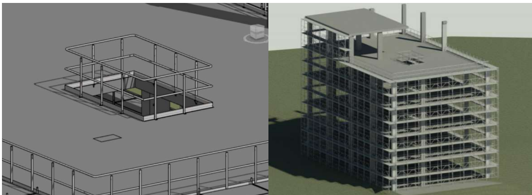
Figure 19: Introduction of the CPE models in real construction BIM model. Source: Alcalde, Gerard [62].
