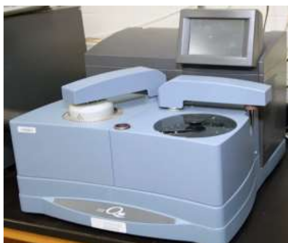
Figura 16: Equipo DSC Q100 V9.9 Build 303. Fuente: Differential Scanning Calorimeter (DSC) TA Instruments Q100 – Wisconsin Centers for Nanoscale Technology – UW–Madison
