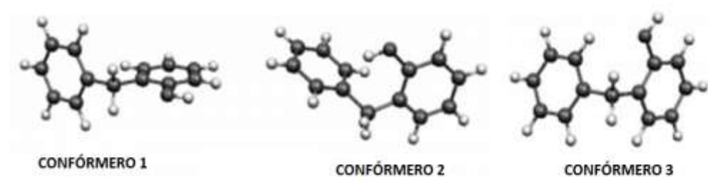
Figura 18: Confórmeros del 2-bencilfenol. Fuente: [13] 1. Katsyuba, S., Chernova, A. i Schmutzler, R. Vibrational spectra and conformational isomerism of calixarene building blocks: 2-benzylphenol . A: Organic and Biomolecular Chemistry . 2003, Vol. 1, núm. 4, p. 714-719. ISSN 14770520. DOI 10.1039/b211164k.
