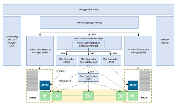
Fig. 1. METRO-HAUL Control, Orchestration, and Management system and network, compute, and storage infrastructure
