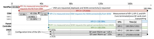
Fig. 7. Service set-up times (KPI-1..3) of different stages of the demonstration.
