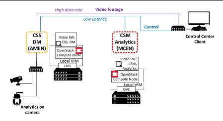
Fig. 2. Video surveillance scenario. Multiple cameras are connected an AMEN node. Analytics and management are performed at MCEN.
