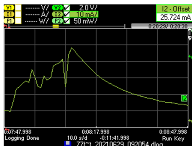
Figure 5. Current consumption pattern of a RockBLOCK Mk2 device that is initially in sleep state, performs an unsuccessful message transmission attempt, and returns to sleep state.
