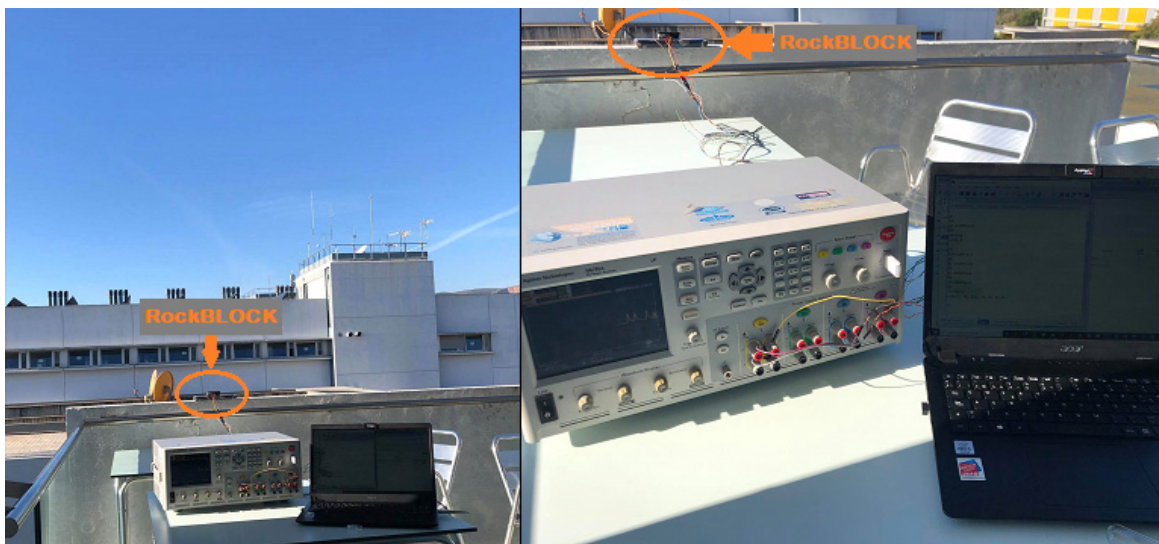
Figure 3. Outdoor scenario used for the current consumption measurements of the RockBLOCK Mk2 Iridium IoT device.
