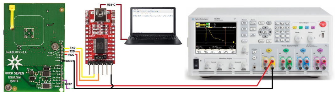
Figure 2. Experimental setup for measuring the current consumption of the RockBLOCK Mk2 Iridium IoT device.
