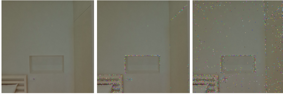
Figure 6.1: An image of a bedroom wall with maximum of 1000 detected keypoints using SIFT. Contrast threshold used, from left to right: 0.1, 0.01, 0.001. [Source: Compiled by author ]
