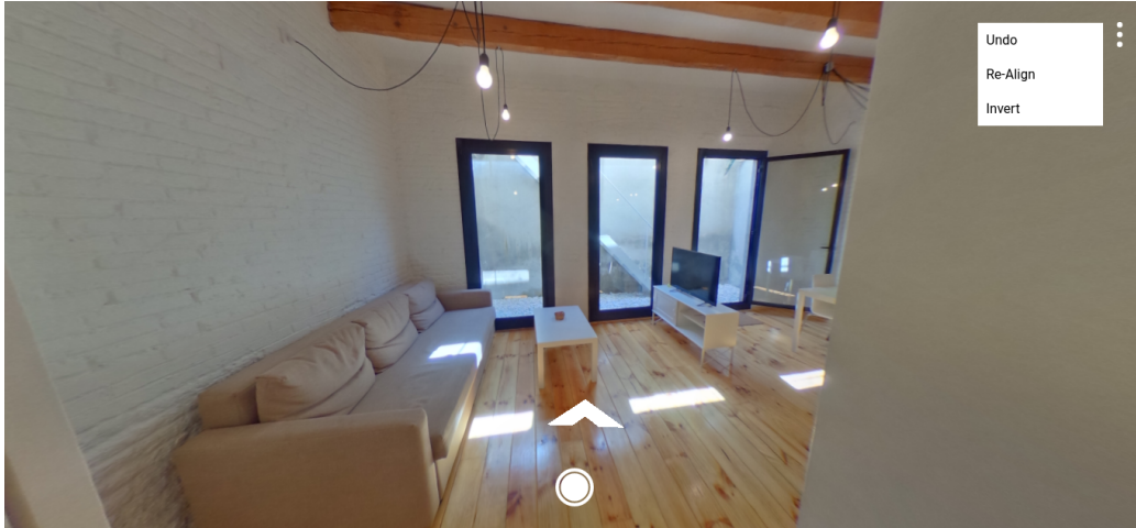
Figure 8.2: 360 Navigator using the reconstructed model. Center: equirectangular image visualiser and adjacent camera location visualiser. Top-right: reconstruction edit controls. Bottom-center: button to add images and connect to the current one. [Source: Compiled by author ]
