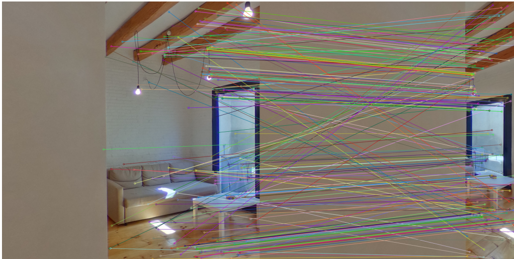
Figure 6.5: Visualisation of matches after essential matrix estimation. Top: non-normalised keypoint coordinates. Bottom: normalised keypoint coordinates. [Source: Compiled by author ]
