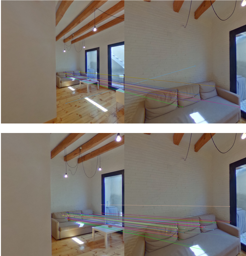
Figure 6.3: Visualisation of matches obtained from (top) not focused regions (154 matches), i.e, having the same FoV, and (bottom) having approximate focus on the same object (239 matches). The matches are filtered without essential matrix error correction. [Source: Compiled by author ]
