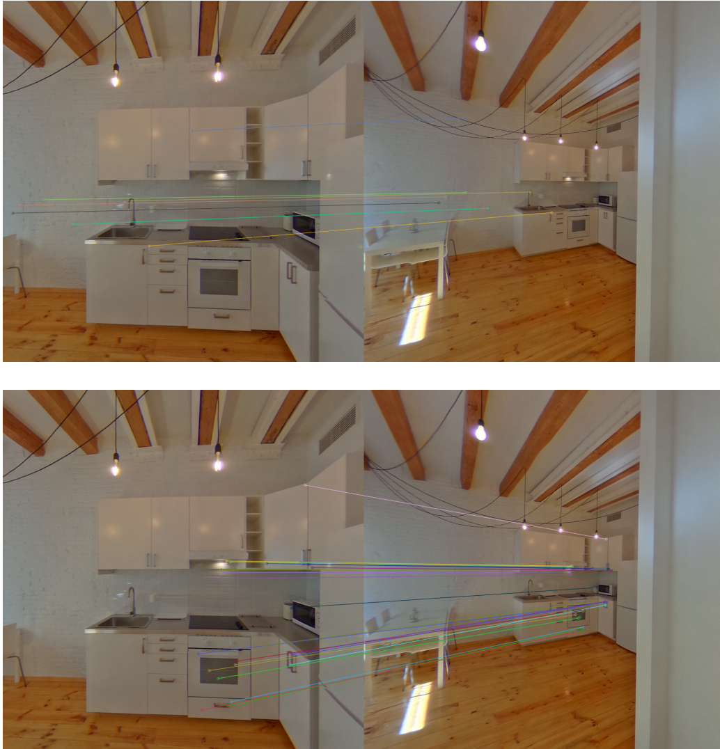
Figure 6.2: Visualisation of matches obtained from keypoints detected with (top) SIFT and (bottom) ASIFT. [Source: Compiled by author ]
