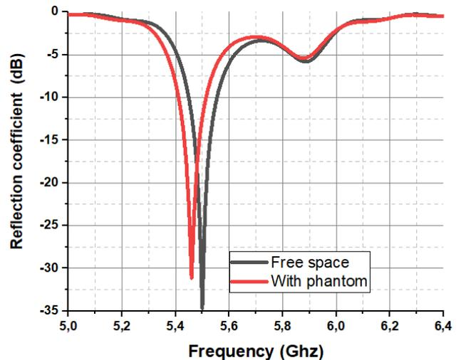
Fig.3. Simulated reflection coefficients of the antenna in free space and on human body equivalent phantom.
