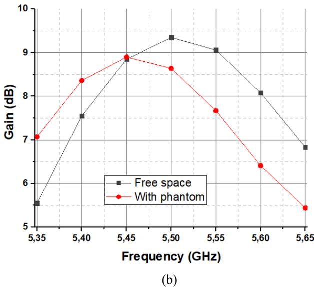
Fig. 6. (a) Efficiency, (b) Gain of the proposed antenna.
