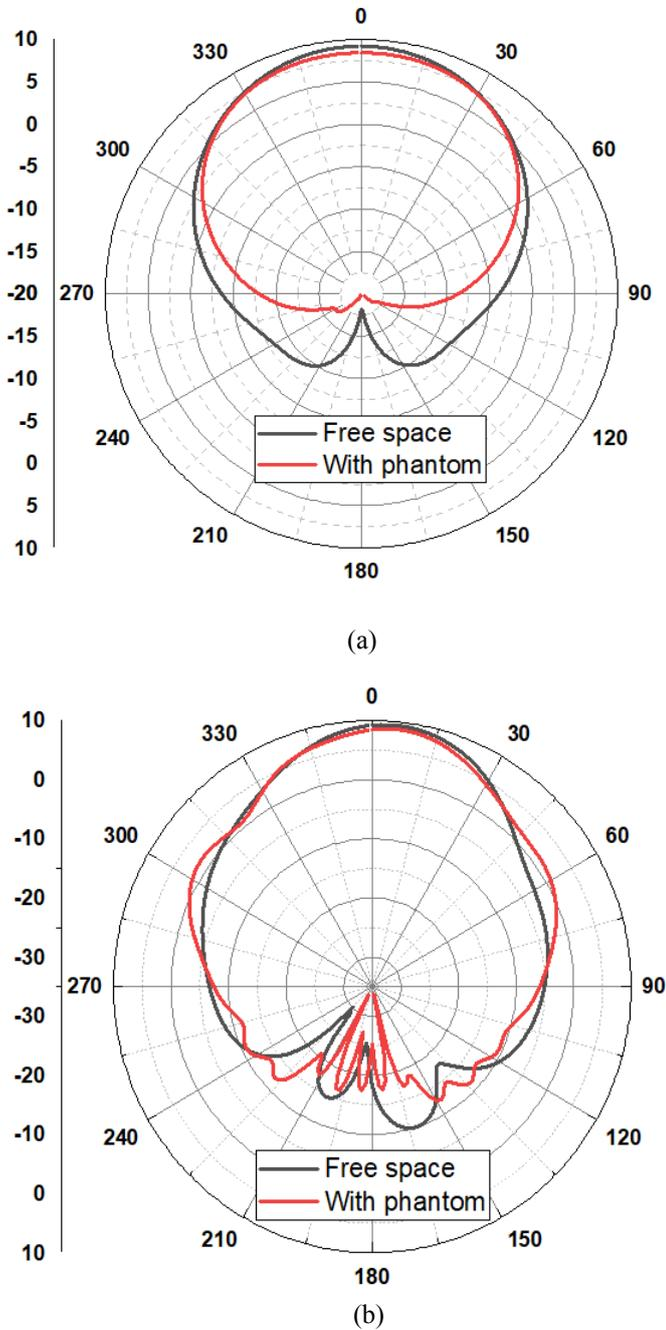
Fig.4. Simulated radiation pattern at 5.5GHz: (a) Electric field plane (E-Plane); (b) Magnetic field plane (H-Plane).
