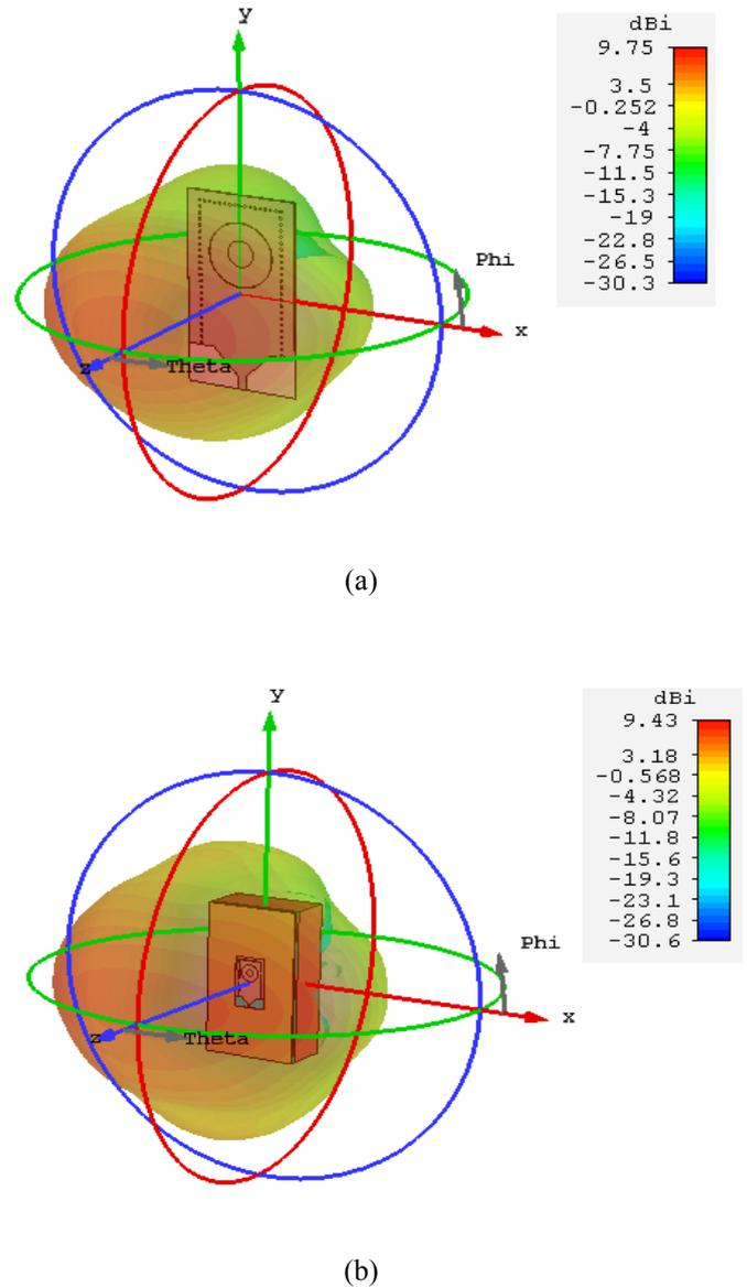
Fig. 5. 3D radiation pattern for the proposed antenna at 5.5GHz: (a) Free space, (b) with phantom.
