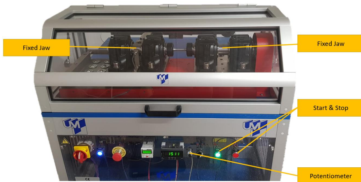
Figure 17: UMI fatigue machine
