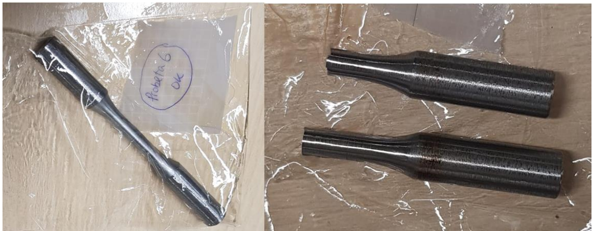
Figure 18: Fatigue specimens (uncycled left, cycled right)
