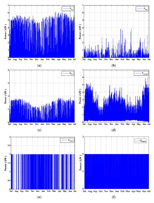
**Figure 2.** Microgrid power profiles: (a) Photovoltaic power, (b) wind turbine power, (c) solar thermal collector power, (d) domestic load demand, (e) electric water heater power, and (f) domestic hot water equivalent power.
