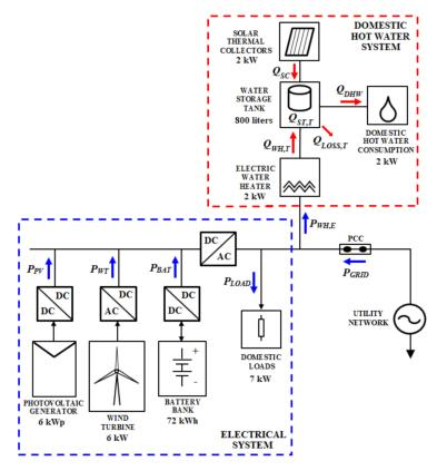
Figure 1. Electro-thermal microgrid architecture.
