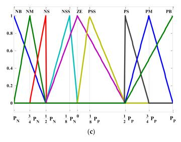
**Figure 4.** Fuzzy controller membership functions (MF): (a) Power forecast error, (b) battery state-of-charge (SOC), and (c) fuzzy logic control (FLC) output [45]. ©2016 IEEE, Reprinted, with permission, from Arcos-Aviles D, Guinjoan F, Marietta MP, Pascual J, Marroyo L, Sanchis P. Energy management strategy for a grid-tied residential microgrid based on Fuzzy Logic and power forecasting. IECON 2016—42nd Annu. Conf. IEEE Ind. Electron. Soc., Florence, Italy: IEEE; 2016, pp. 4103–4108.
