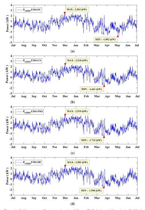
**Figure 9.** Grid power profile comparison for different EMS designs (**a**) heuristic, (**b**) CS algorithm, (**c**) PSO, and (**d**) DE algorithm.
