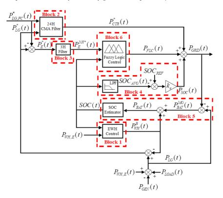
**Figure 3.** Energy management strategy block diagram [43]. ©2018 IEEE, Reprinted, with permission from D. Arcos-Aviles et al., "Fuzzy-based energy management of a residential electro-thermal microgrid based on power forecasting," in IECON 2018—44th Annual Conference of the IEEE Industrial Electronics Society, Washington, DC, USA, October 2018, pp. 1824–1829.
