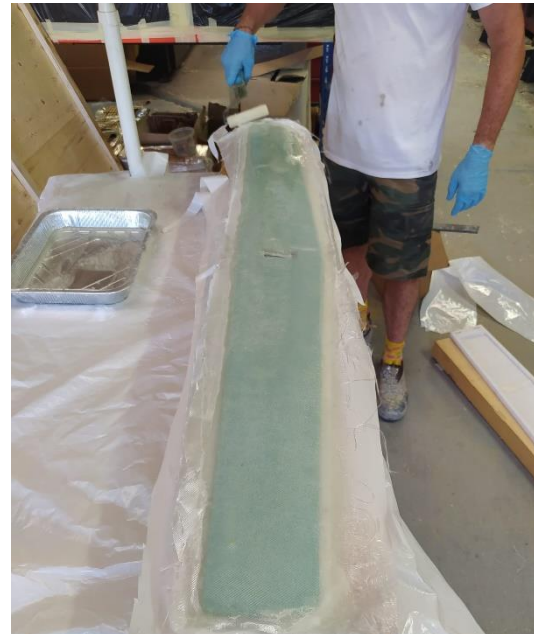
Figure 66: hand lay-up process over the foam core.
