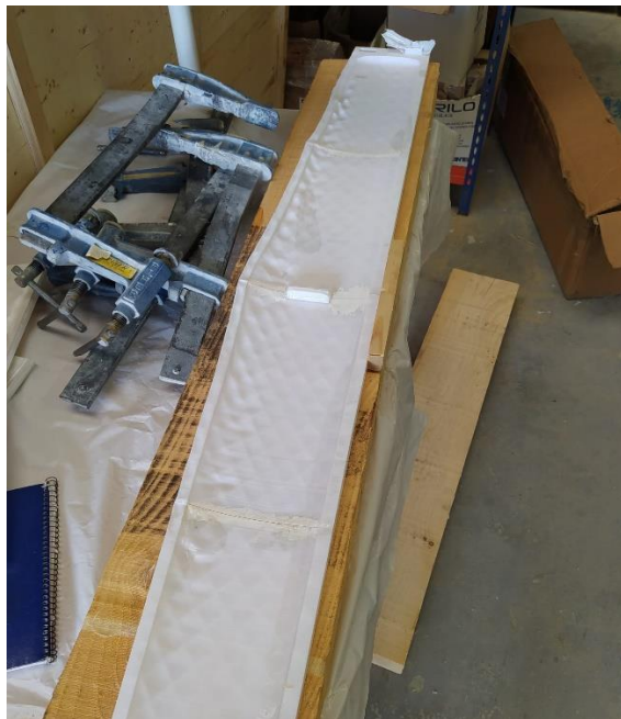
Figure 70: deformities of the lower mould.
