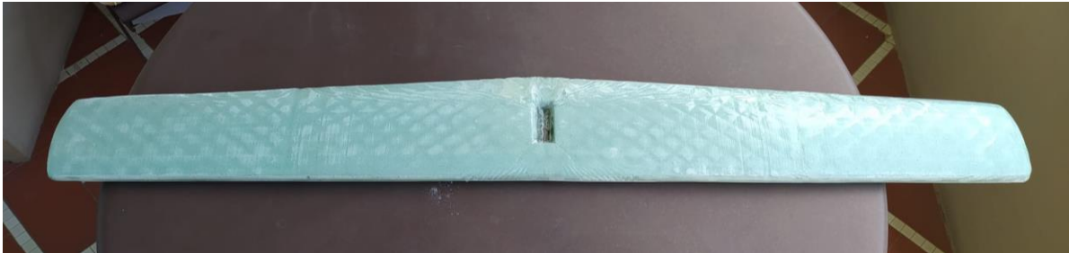
Figure 71: finished centreboard foil prototype.
