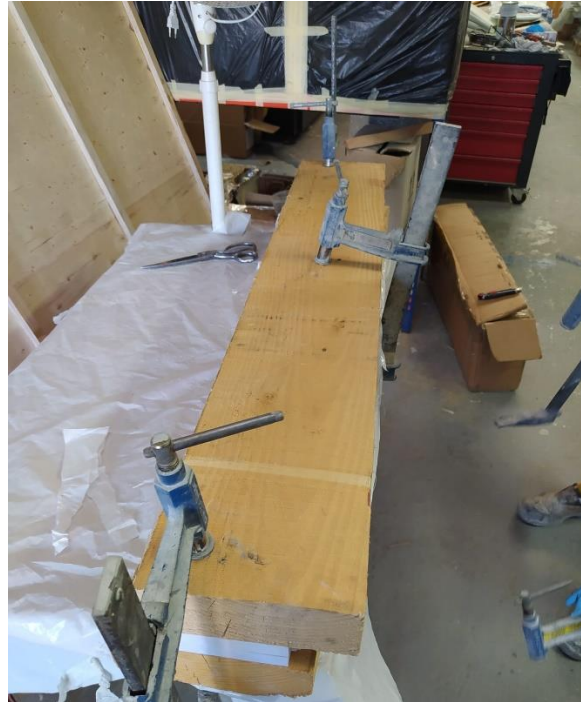
Figure 68: closed moulds with applied pressure.
