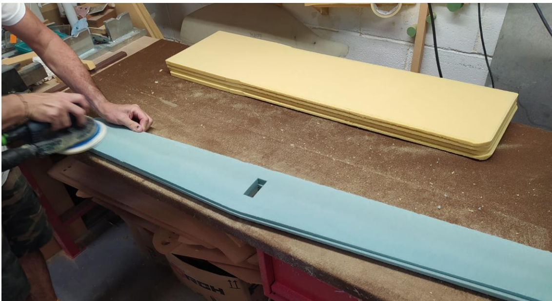
Figure 64: trimming of the foam core.
