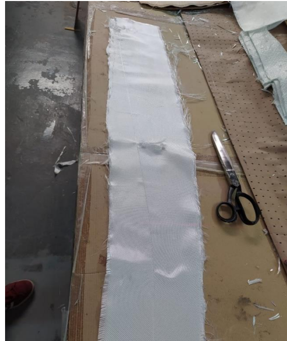
Figure 63: CNC cutting the E-glass fibre fabric.
