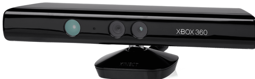
Figure 4.6: A Kinect camera, used to capture RGB-D images and obtain current mesh positions
