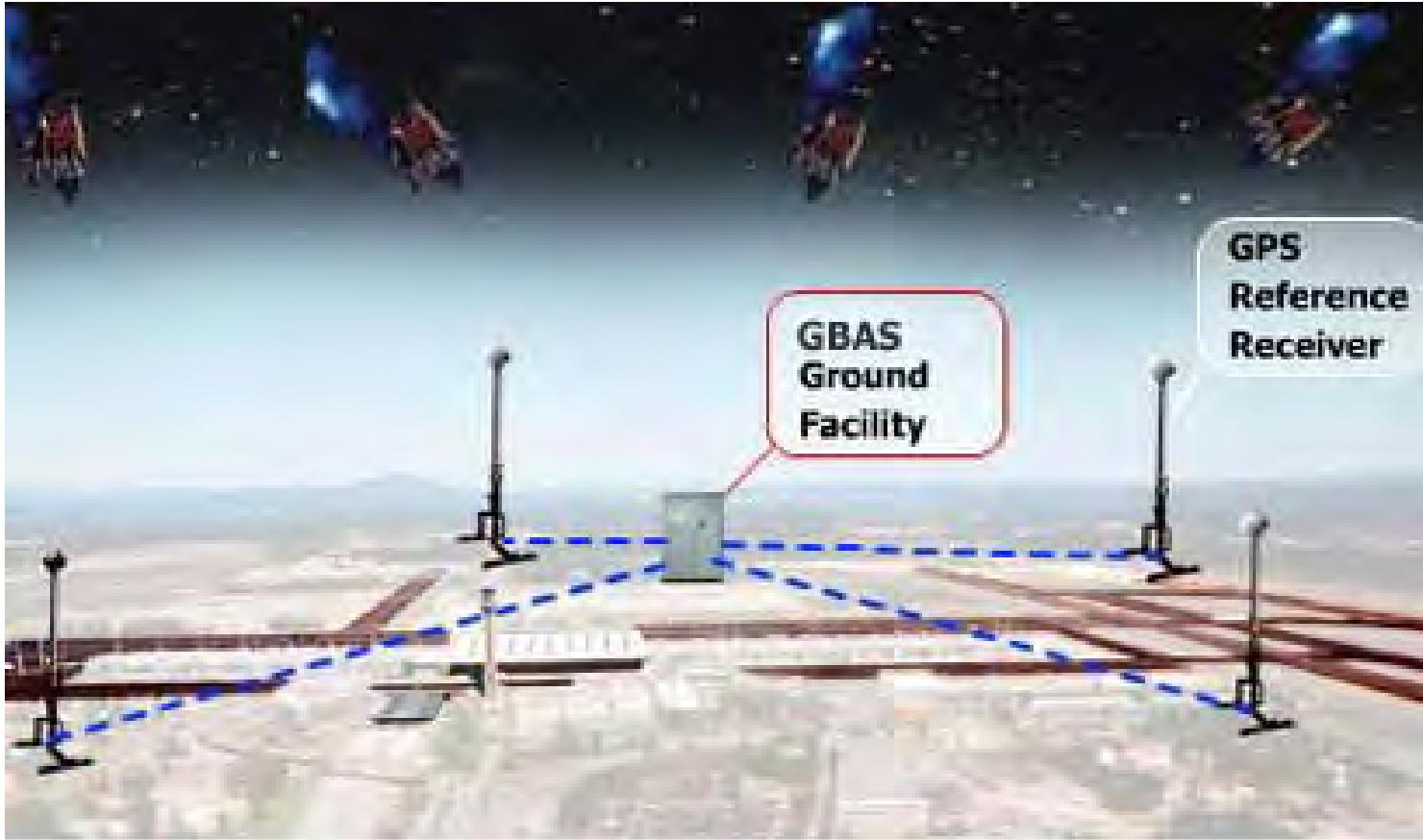
**GBAS Ground Facility (LGF) Calculates Errors in GPS Position and Formulates the GBAS Correction Message**
