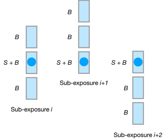
**Fig. A.1.** Schematic illustration of the default MSA observing scheme where each target is assigned a three shutter tall slitlet, and the telescope is nodded between subexposures such that the target is cycled between the three shutters of the slitlet.
