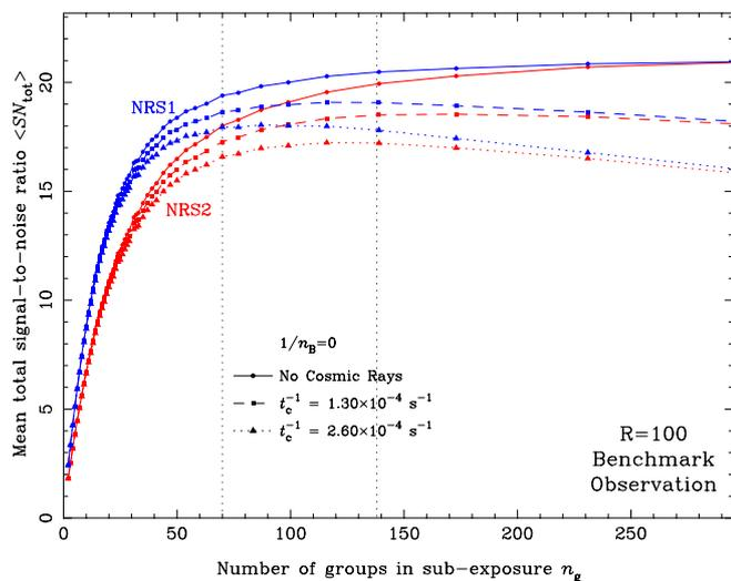
**Fig. A.5.** Mean total signal-to-noise ratio achievable in the benchmark  $R = 100$  continuum detection case for a fixed total exposure time of  $t_{\text{int}} = 10^4$  s as a function of the number of  $n_g$ ,  $m = 1$  groups in each subexposure.
