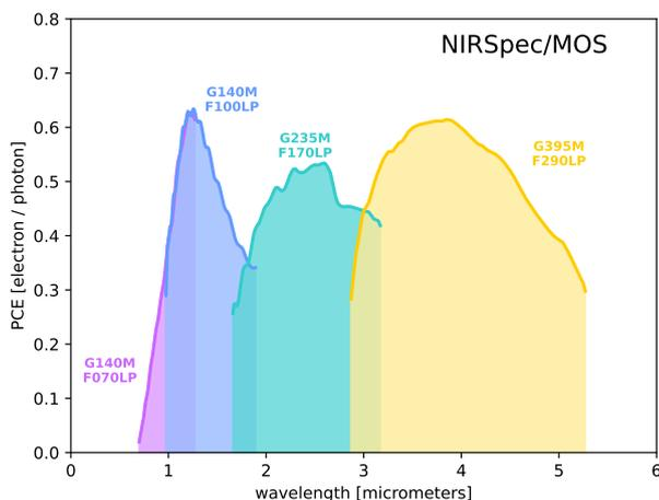
**Fig. 8.** Photon conversion efficiency of NIRSpec as a function of wavelength when employing the three  $R = 1000$  gratings and their order-separation filters.
