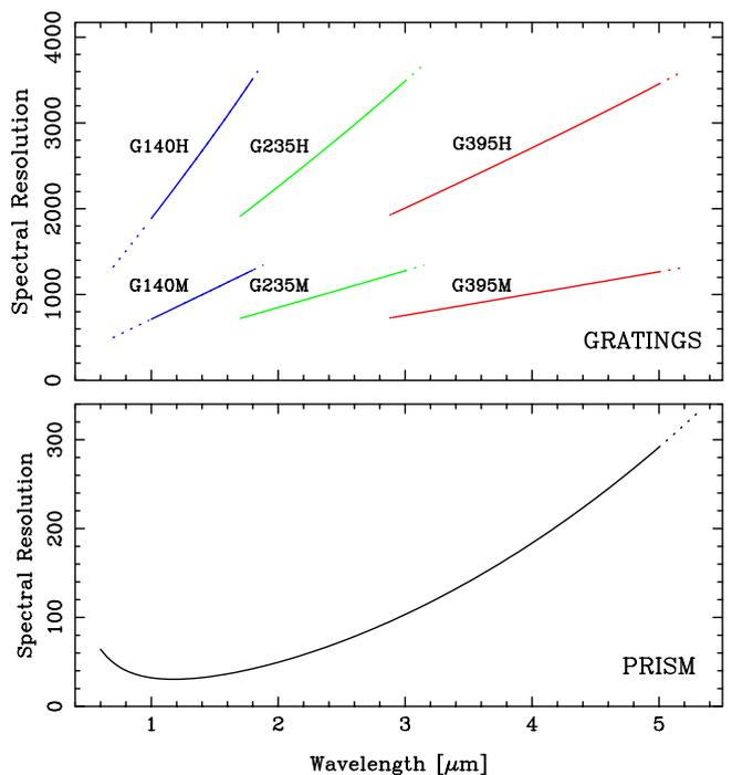
**Fig. 5.** Wavelength ranges and spectral resolutions achievable with the seven dispersers of NIRSpec. The nominal wavelength range covered by each disperser is shown as a full line, and the anticipated actual usable range as a dotted lines, including the blue extensions of the G140M and G140H gratings when used with the F070LP filter.
