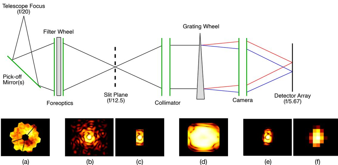
**Fig. 10.** Schematic of the optical chain of NIRSpec showing Fourier optical simulations of the expected Point Spread Function and beam footprint in the two pupil and focal planes of the system (see text). The simulations refer to a monochromatic point source at a wavelength of  $\lambda = 2\mu\text{m}$ . A logarithmic look-up table is employed in order to show the full range of the light distributions.
