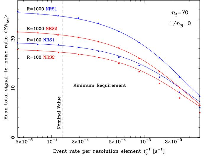
**Fig. A.4.** Mean total signal-to-noise ratio achievable in the two benchmark observations when employing NRSIRS2RAPID subimages spanning  $n_g = 70$ ,  $m = 1$  groups plotted against the incident cosmic ray event rate in a resolution element. The triangles and squares mark the outcomes of matching Monte Carlo simulations
