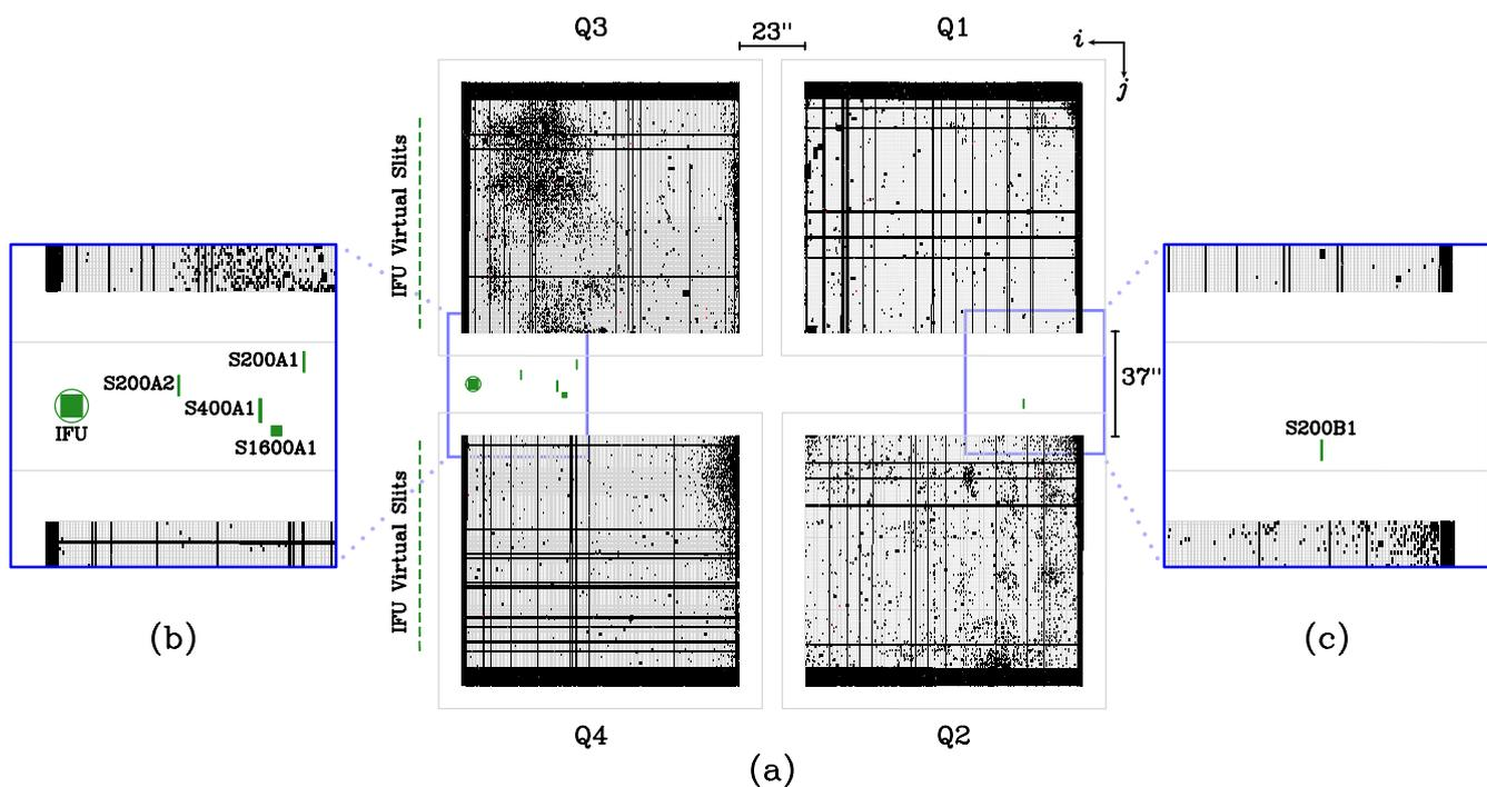
**Fig. 4.** Layout of the NIRSpec Slit Plane. (a) The four quadrants of the Microshutter Array, the five Fixed Slits, the entrance aperture of the Integral Field Unit, and the locations of its 30 virtual slit images. The dispersion direction is horizontal. Black areas in the MSA depict inoperable vignettted or permanently closed shutters. (b) Close-up of the left-most group of four Fixed Slits and the IFU entrance aperture. (c) Close-up of the right-most redundant Fixed Slit.
