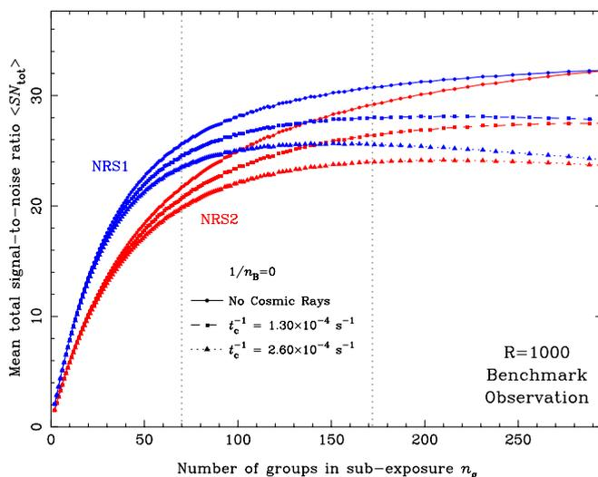
**Fig. A.6.** Mean total signal-to-noise ratio achievable in the benchmark  $R = 1000$  emission line detection case for a fixed total exposure time of  $t_{\text{int}} = 10^5$  s as a function of the number of  $n_g$ ,  $m = 1$  groups in each subexposure.
