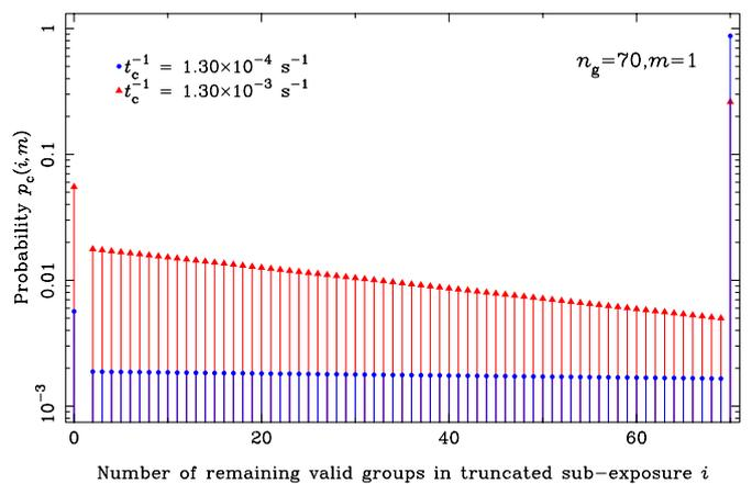
**Fig. A.3.** Probability that an exposure ramp extending over  $n_g = 70$ ,  $m = 1$  groups runs to  $\tilde{n}_g = i$  valid reads before the resolution element spanning 8 detector pixels is hit by a cosmic ray. The blue circles are for the nominal assumed cosmic ray incidence rate. The red triangles are for a ten times higher event rate. Note the logarithmic ordinate scale.
