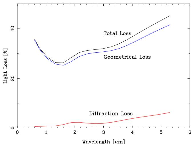
**Fig. 11.** Fourier optical prediction for the total slit loss experienced by a point source perfectly centered within a single shutter of the MSA as a function of wavelength. The geometrical loss caused by the truncation of the point spread function by the open area of the shutter and the subsequent diffraction loss caused by light in the spread-out beam missing the disperser are shown individually.
