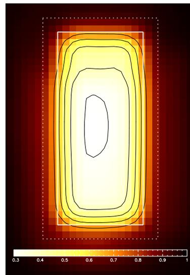
**Fig. 12.** Fourier optical prediction for how the total slit loss from a point source varies with its placement within a single shutter at a wavelength of  $\lambda = 2.0\mu\text{m}$ . The shutter open area and pitch are indicated by the solid and dotted white lines.
