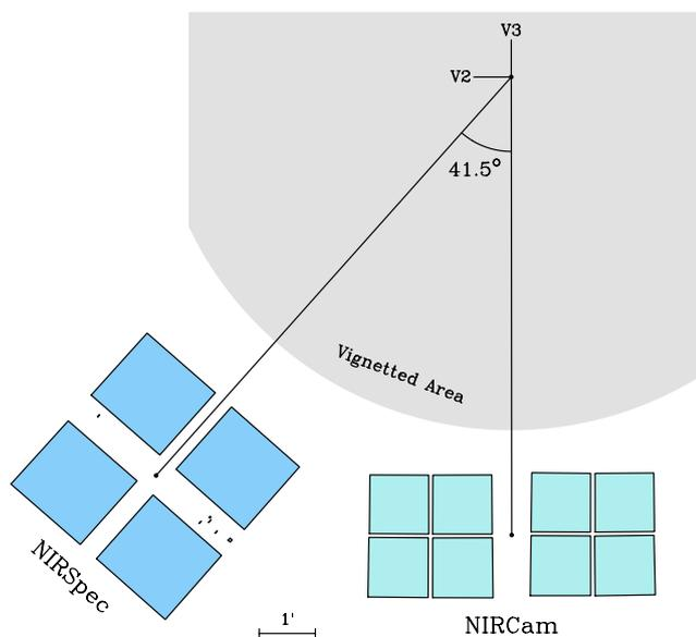
**Fig. 3.** Location and orientation of the NIRSpec field of view on the shared JWST focal sphere with respect to NIRCams and the telescope optical axis. The entrance apertures of the other two JWST instruments, MIRI and NIRISS, are situated to the right of and below NIRCams.
