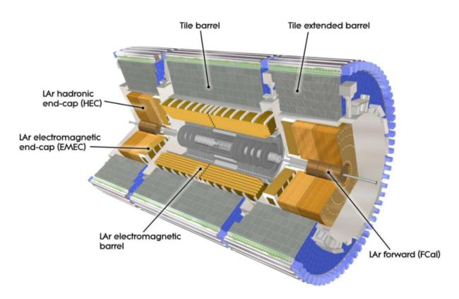
Figure 3.5.: A cut-away view of the ATLAS calorimeter. Figure taken from Ref. [13].
