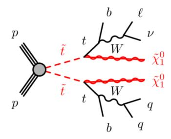
Figure 6.1.: Feynman diagram of the SUSY decay scenario considered for the main analysis presented in this thesis. The *stop* decays to a *top* and a lightest neutralino because  $\Delta m(\tilde{t_1}, \tilde{\chi}_1^0) < m_W + m_b$  as explained in Section 2.4.
