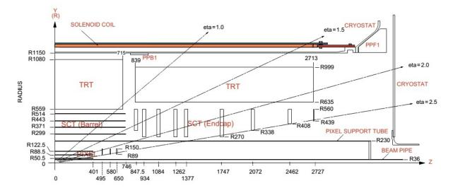
Figure 3.3.: A cross-section taken parallel to the beam pipe of one quadrant of the SCT and its positioning relative to the PIXEL Detector and TRT. The positions of the barrel layers (horizontal lines) and end-cap disks (vertical rectangles) are shown in radial and longitudinal coordinates, with their exact coordinates labelled. Various values of  $\eta$  are shown for orientation. Figure taken from Ref. [91].
