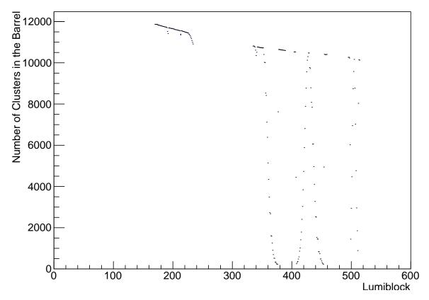
Figure 4.12.: Number of clusters vs. lumiblock for the barrel region of the SCT for the  $\mu$ -scan run taken in Run 280520 calibration pixel beam stream.
