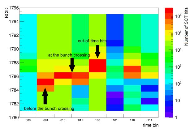
**Figure 4.11.:** SCT timing information for BCIDs surrounding the BCID of the collision at 1786 (Run 266904 calibration pixel beam stream).
