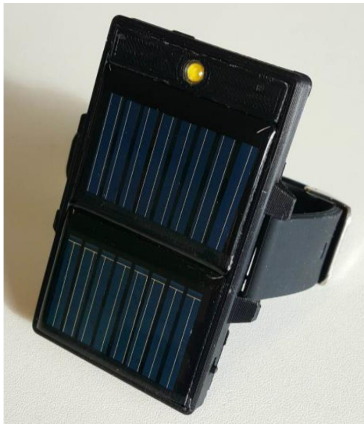
Figure 4.6. Prototype of the Solaware wearable wrist solar-powered lighting device. (Source: Solaware)
