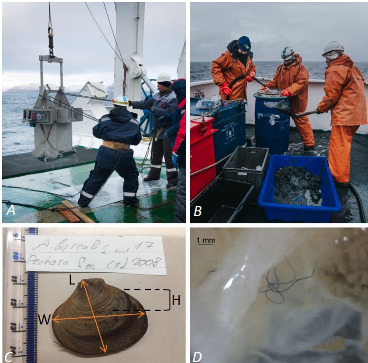
Fig. 4.3 - 2. Overview of methods of microplastic sampling (A) Deployment of the box corer onboard expedition AMK-78, photo courtesy of Vyacheslav Volodin; (B) Washing of the sediments, photo courtesy of Anastasia Zagovenkova; (C) Schema of morphometric measurements of the bivalve mollusc Astarte borealis , L – length; W – width; H – height; (D) Microplastic fibre inside the mantle cavity.
