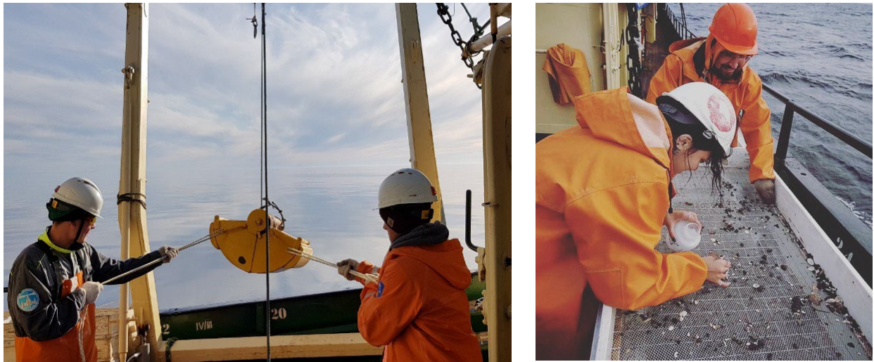
Fig. 2.3 - 3. Deployment of the benthic grab Okean-50 during the RV Kartesh expedition in 2018 (on the left); washing of the sediments from the grab over the upper mesh (5 mm) of the washing table in 2016 (on the right). Photo courtesy of the LMSU MRC.
