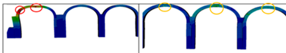
Fig. 22. (a) Deformation shape of first (west) span after a 100 kN horizontal point load has been applied on the right hand-side abutment, (b) Deformation shape of fourth, fifth and sixth spans after a 100 kN horizontal point load has been applied on the right hand-side abutment.
