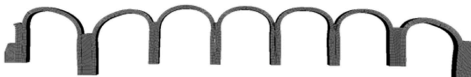
Fig. 25. Deformation shape of the structure after a 100 kN horizontal point load has been applied on the further left hand-side abutment together with a 100 mm vertical displacement on the 100 mm vertical displacement of the second and eighth support.
