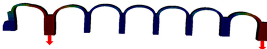
Fig. 23. Deformation shape of the structure after 100 mm vertical settlement of supports 2 and 8.
