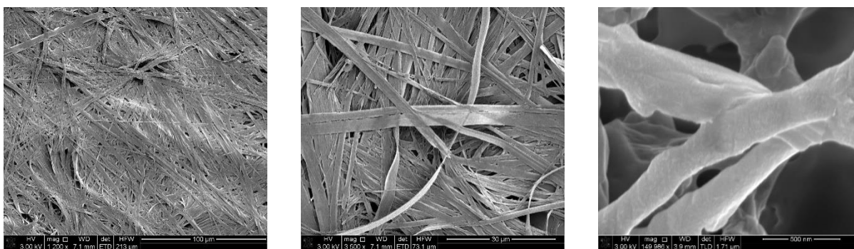
Figure 6.11: SEM micrographs of the dried xerogel of 1 aniline at 1 wt%.
