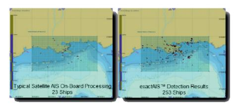
Figure 2 - The difference between standard AIS signals (left) and satellite exactAIS signals (right) [24]
