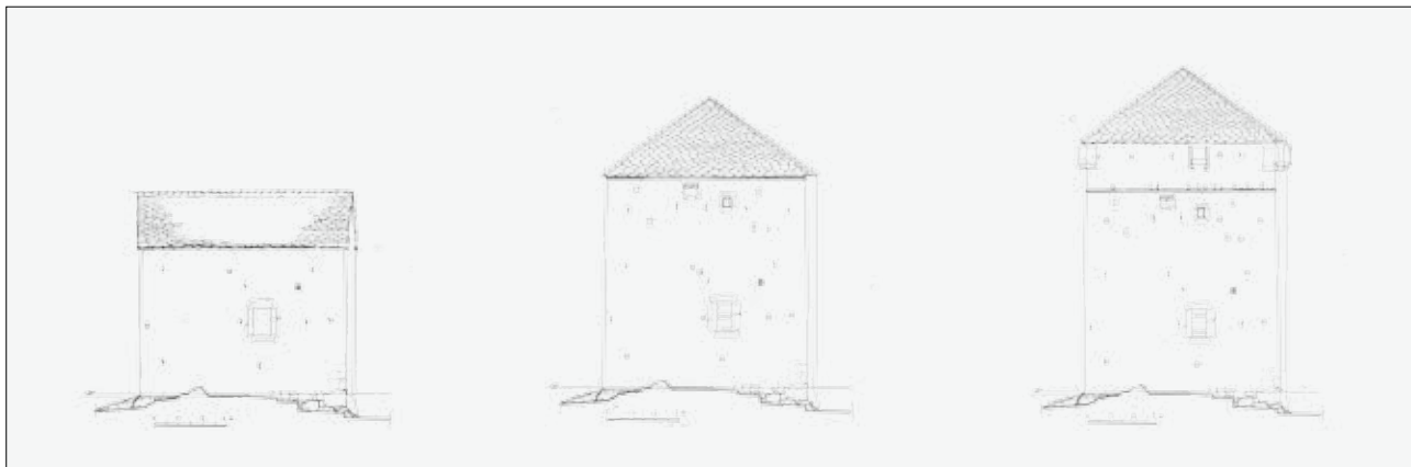
8 Zalina kula, jugozapadno pročelje, tri faze prostornog razvoja kule (crtež: A. Gamulin, 2020.) Zalina tower, southwest façade, three phases of spatial development (drawing: A. Gamulin, 2020)
