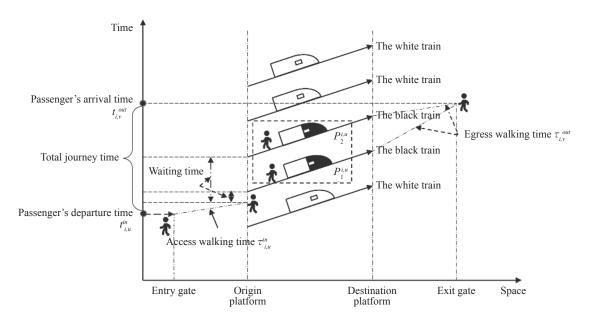
Figure 1 – Possible passenger-and-trains matching
