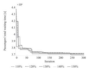
Figure 11 – The comparison of optimisation results under different full-loaded coefficients of a train
