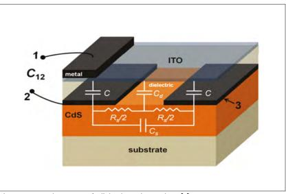
Figure 5. Internal structure of a light-dependant resistor [9]
