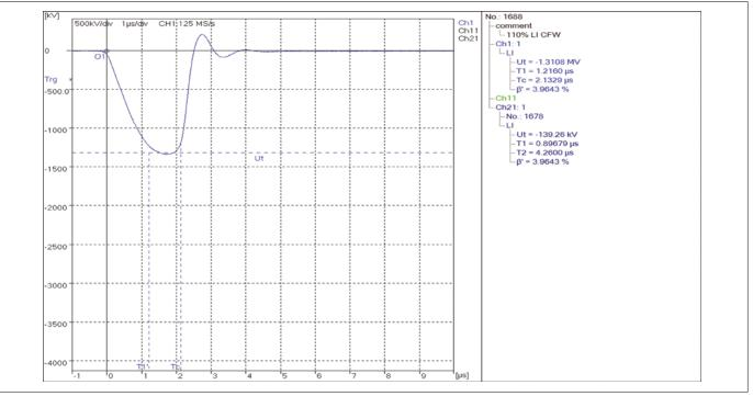
Figure 19. A typical profile for an applied high voltage impulse in EMI tests
