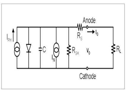
Figure 6. An electrical model for photodiodes [10]
