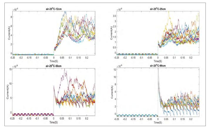
Figure 12. The distance effect on the light sensitivity of photodiodes
