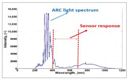
Figure 3. The light intensity of a 100 kHz electric arc at different voltage-wavelength [8]
