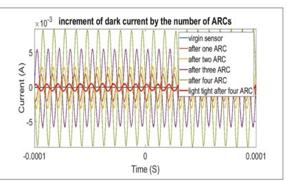
Figure 25. Increment of the dark current after each arc for the photoresistors
