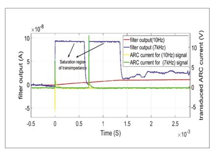
Figure 11. The effect of filtering on the output signal
