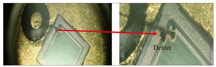
Figure 24. The substrate of a photodiode with certain defects due to proximity to the electric arc
