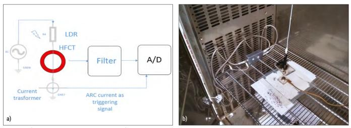
Figure 10. a) A schematic of the measuring circuit b) A part of the setup used for LDRs
