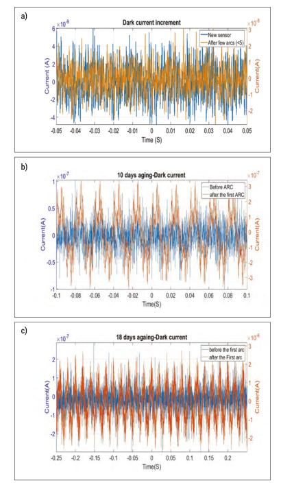
Figure 22. The effect of thermal ageing in oil on the amount of dark current: a) unused sensor b) after ten days ageing c) after 18 days ageing
