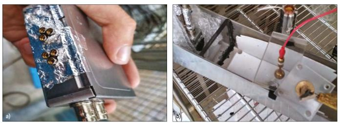
Figure 9. Some parts of the measuring circuit as for photodiodes a) Two pairs of photodiodes in a shield box, b) The measuring chamber
