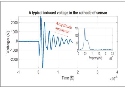
Figure 4. Potential of the cathode in a photodiode adjacent (12 cm) to a 50 Hz electric arc at the time of arc formation
