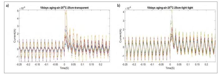
Figure 23. a) the output signals for a transparent sensor after 18 days ageing, b) corresponding signals for a light-tight sensor
