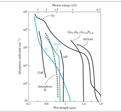
Figure 1. The absorption coefficient of some materials with respect to the wavelength and photon energy [3]
