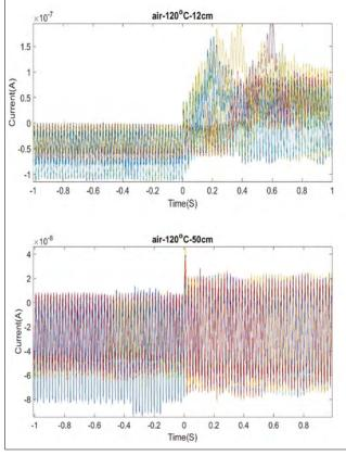
Figure 16. The temperature effect on the performance of photodiodes
