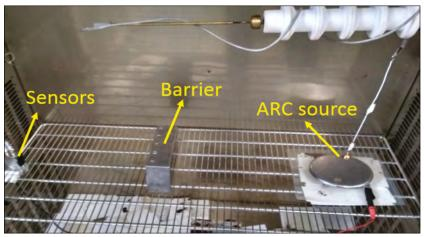
Figure 17. A typical configuration for the barrier effect
