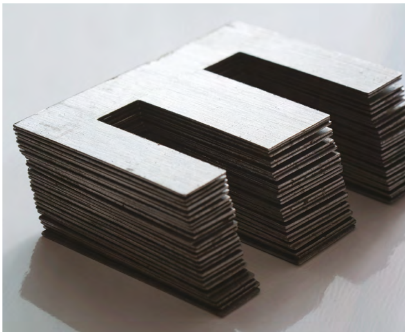
Figure 3. Transformer magnetic steel laminates
