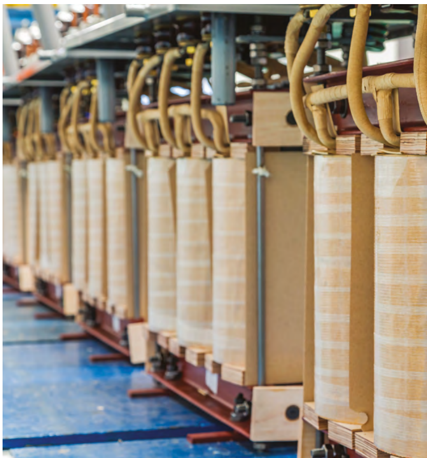
Figure 1. Coils in the production line of three-phase oil-filled distribution transformers
