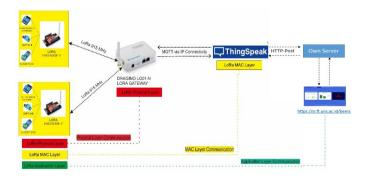
Fig. 1. Proposed system architecture hardware
