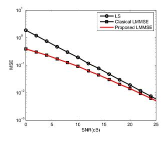
Fig. 1. MSE vs SNR performance comparison of proposed LMMSE, classical LS and LMMSE channel estimator
