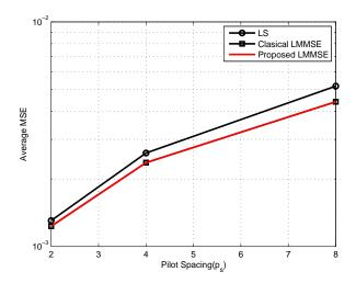
Fig. 3. MSE vs pilot spacing of proposed LMMSE, classical LS and LMMSE channel estimator
