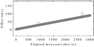
Fig. 1. An offset-set between a measurer and a device that are connected through a wired network.
