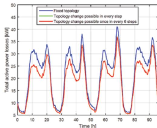
Fig. 4. Total active power losses during all three simulation runs in the scenario 1.
