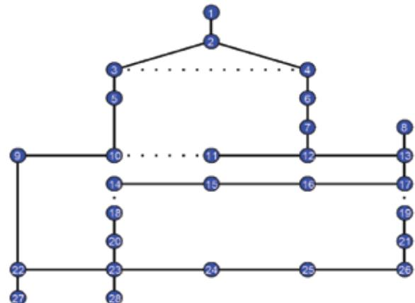
Fig. 1. Graph representation of the distribution grid in Koprivnica.
