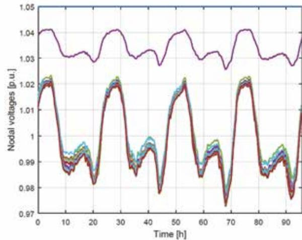
Fig. 3. Nodal voltage magnitudes during simulation 1.3.
