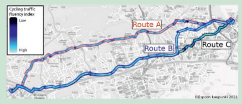
Fluency of three different cycling routes between Otaniemi and Kivenlahti in Espoo. Route C is the shortest and Route A the fastest according to the dataset, but Route B offers the most fluent cycling experience.
