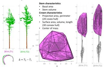
Figure 1. Illustration of the tree characteristics derived from the classified point clouds.
