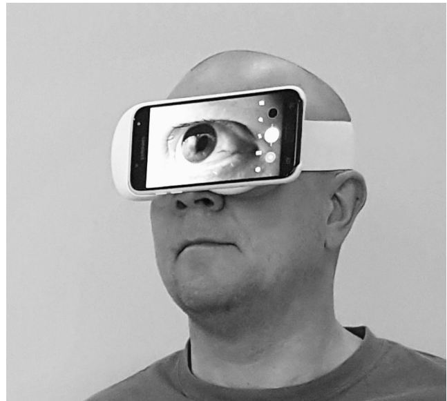
FIGURE 1 Mobile phone attached to specifically designed goggles was used to record eye movements after cold water swimming legs
