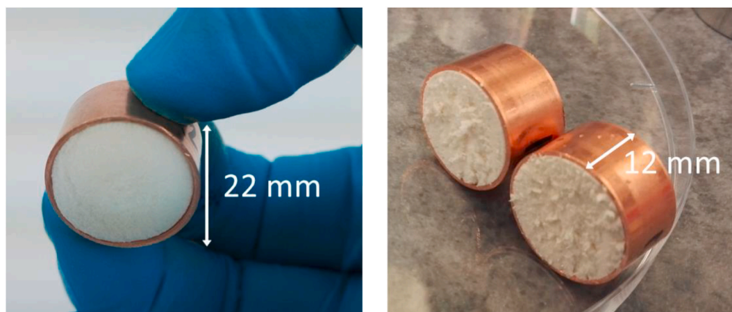
Fig. 5. Prepared nanofoams (MCB_0.3 on the left image and MCB_0.75 on the right) mounted in copper bush rings.
