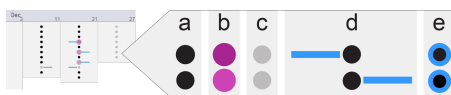
Figure 2: Various states of the dots inform users about the exploration process (R1). Each dot represents an item in the collection. (a) Dots that have not been selected yet; (b) dots under selection. The more saturated colour represents the more recently selected items; (c) dots that have been selected and pushed out of the stack of the snippet view; (d) and (e) the blue marks indicate relationships that can be visually overlaid with the other three states. They depict item relations to the currently focused categorical facet value; in the case of emails, (d) affords contact relations where the left-side line indicates a sender relation and the right-side line denotes a co-recipient relation; (e) denotes keyword relations.
